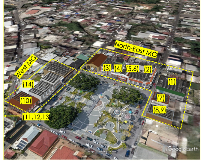
Fig. 1. Initial 3D render of two MGs in Adjuntas, Puerto Rico. Rooftop PV and participating businesses may differ from final installation (Photo credit, Casa Pueblo). Businesses include bakery, pizzeria, furniture stores, hardware stores, optical store, a church and critical facilities such as a pharmacy among others.
