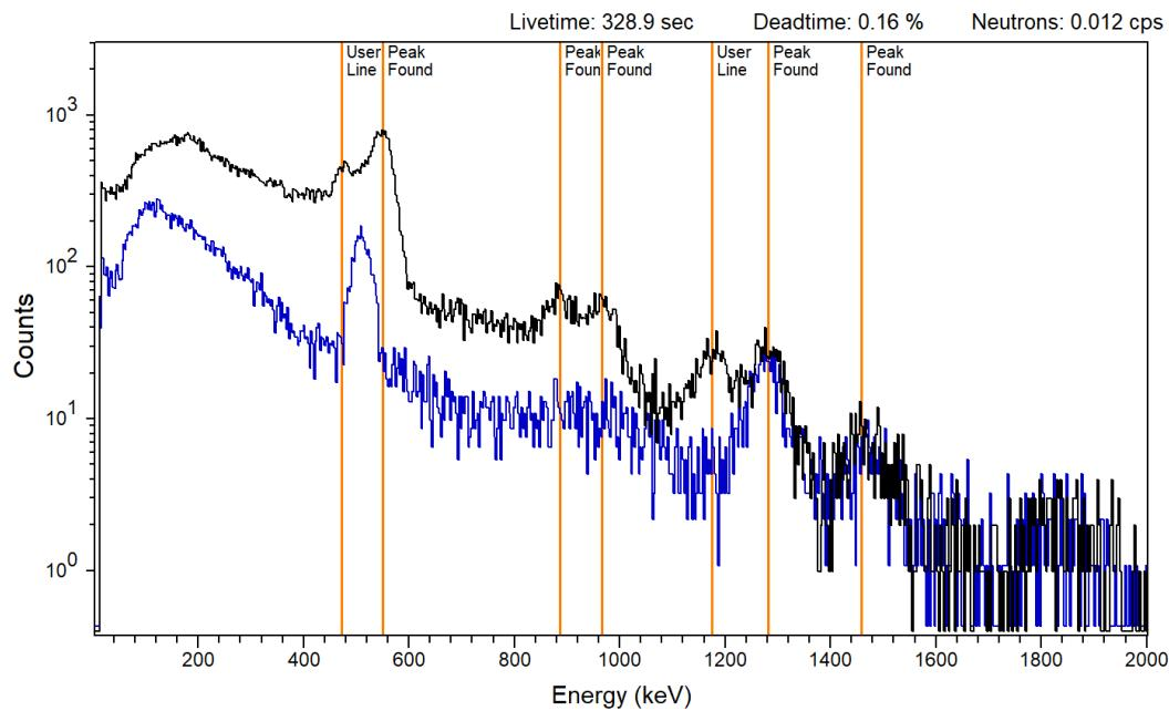
Question 3: Which one of the following radionuclides would be most useful as source of gammas in a  ${}^9\text{Be}(\gamma, \text{n}){}^8\text{Be}$  photoneutron source? The threshold gamma energy for the reaction is 1666 keV. Explain your reasoning. The spectrum "Photoneutron" shown below may be useful for checking your answer. This spectrum was collected at a customs inspection station using a LaBr<sub>3</sub>-based RadSeeker instrument.
