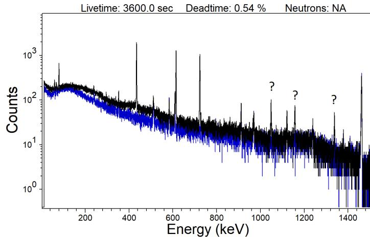
Question 5: A package of aircraft turbine blades is measured with an NaI-based GR-135 instrument after completion of a radiographic inspection. The inspection involved exposure to thermal neutrons.
