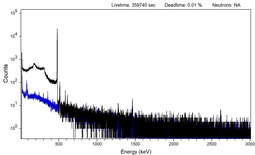
Question 2: The spectrum "Trial Drug" shown below is collected from a shipment of a radionuclide under study for medical applications (targeted radionuclide therapy). The shipment is apparently shielded so that no gamma rays below 450 keV are visible. The spectrum is from a NaI-based RadSeeker detector with an internal Na-22 calibration source. The background, shown in blue, includes the calibration source.
