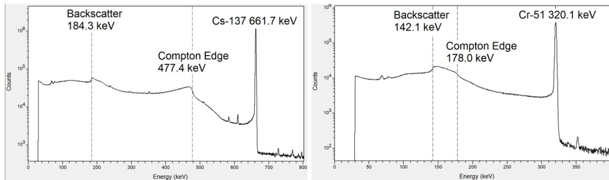
Question 2: The two spectra shown are from two Cs-137 sources with different activities and different amounts of iron (Fe) shielding. Which has the greater amount of shielding?
