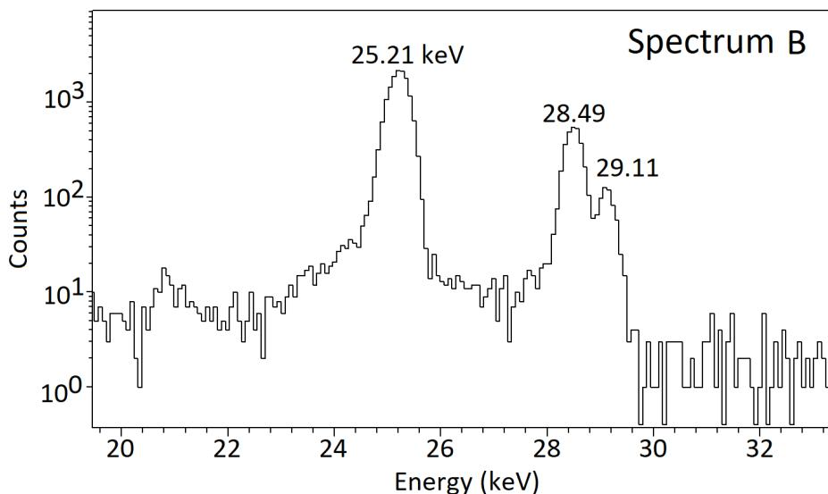
Question 16: The spectra below are collected from highly-enriched uranium (HEU) and Cu-67 using a sodium iodide (NaI) detector. Which spectrum is from HEU?
