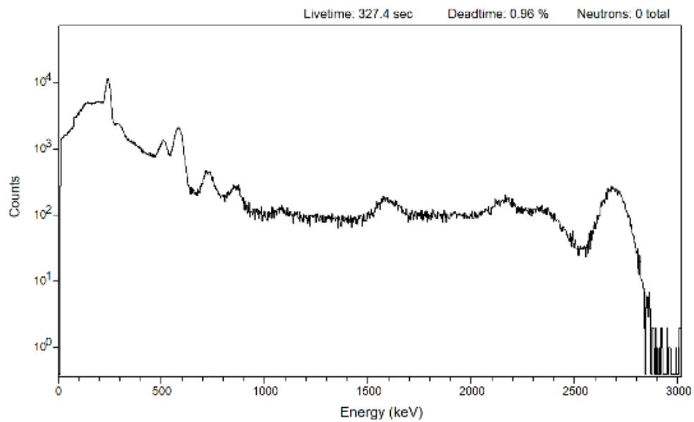
Question 8: The file *Portal.n42* contains a time series of spectra from a Radiation Solutions Model RS-705 spectroscopic portal monitor, which has four 2-inch  $\times$  4-inch  $\times$  16-inch NaI detectors and two Li-6 "Silverside" neutron modules that are linked together. Spectra are recorded once every second while a person walks through the portal. Spectra are available in a linear format (3 keV/channel, "LinEnCal") and also in a format with variable channel width ("CmpEnCal").
