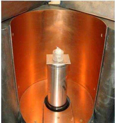
Pellet is in a plastic holder centered on the detector face, separated from detector by 1 mm of plastic.
