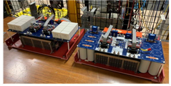
Fig. 9. Single-stage DAB inverter. Transformer is not shown here.
