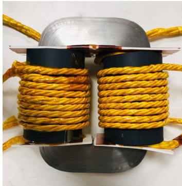
(b) 100kW transformer with L_r/L_m=0.052\%
