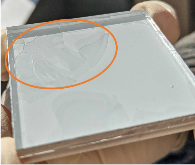
Fig. 12 Optical distortion due to the separation of the light spreader and the scintillator (circled in orange).
