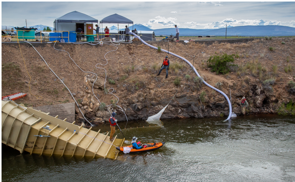
Figure 58: a view from across the canal shows the turbine draft tube (left), control injection station and hose (center), and recovery team in place along the bank and on the water.
