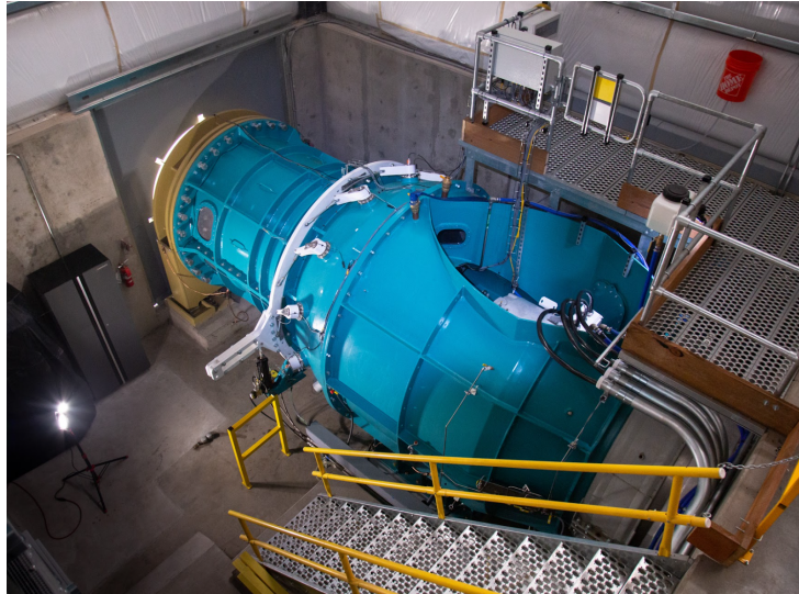
Figure 42: the prototype RHT D190 turbine which was used to conduct the full scale passage tests.
