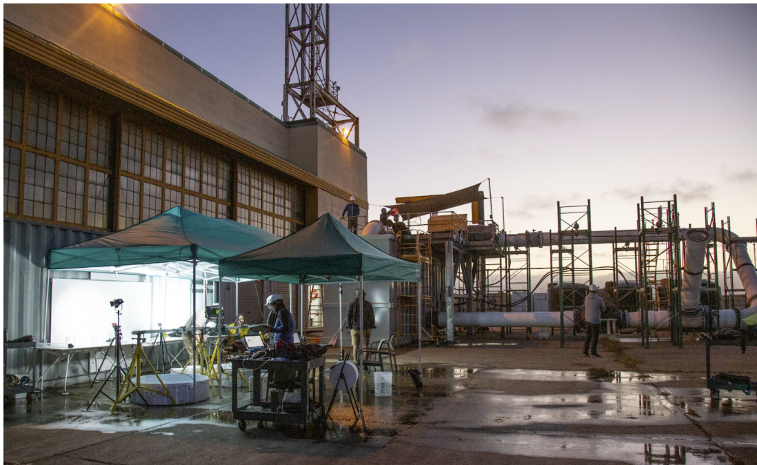
Figure 46: The test facility included a pre- and post-test evaluation area (foreground) and Natel's hydraulic test facility and RHT turbine with injection and recovery apparatus (background).
