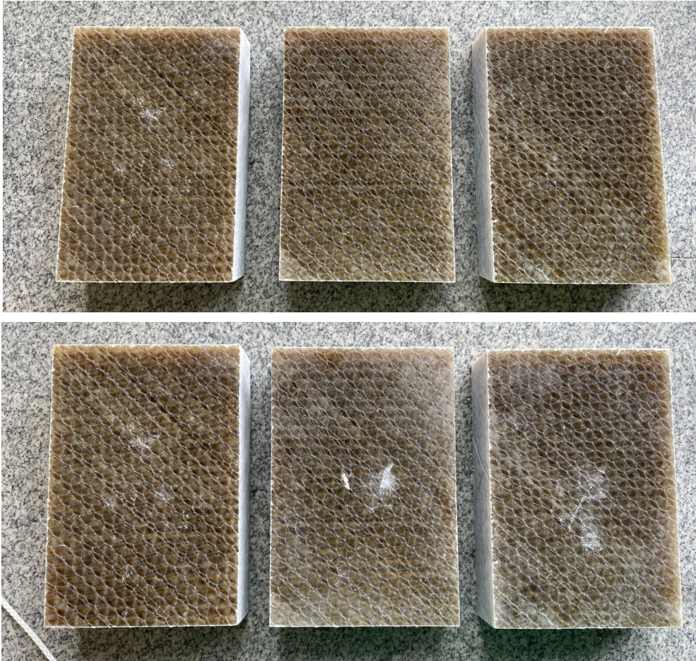
Figure 84: 36 mm thick fiberglass before (top) and after (bottom) impact with concrete impactors dropped from 15 ft.
