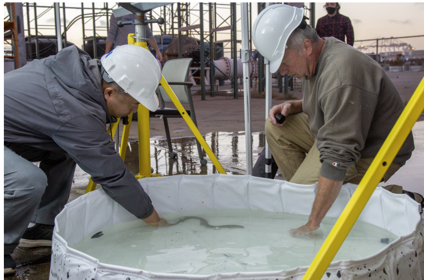
Figure 52: post-test assessment included a behavioral test to assess for lethargy, loss of equilibrium, or other effects in addition to any observable injury.
