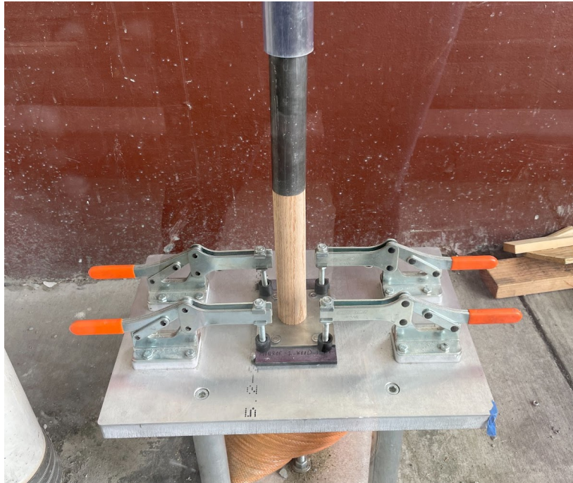
Figure 81: wooden (oak) impactor backed by steel mass set up to impact a carbon fiber coupon.
