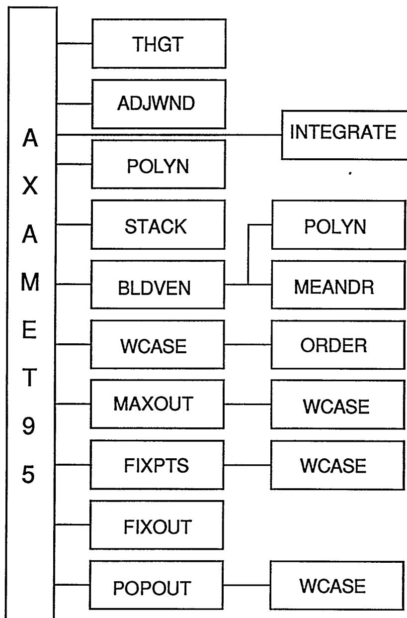
Figure 6. Subroutine Paths for the AXADOS95 Module
