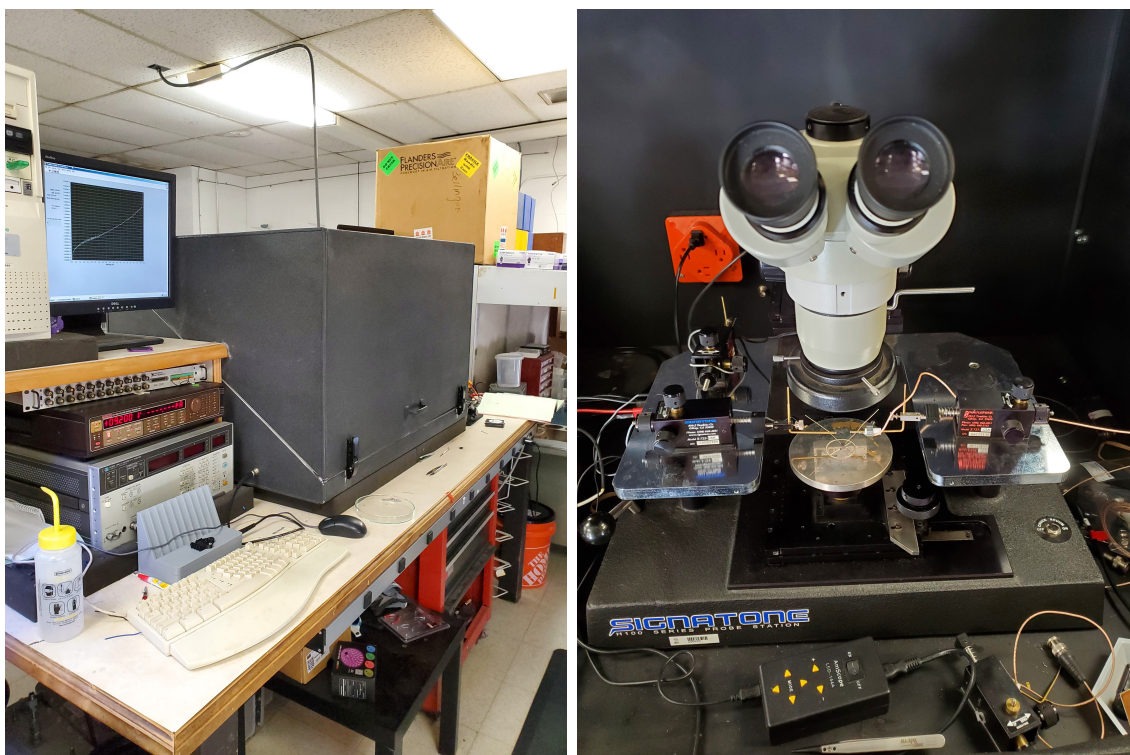
Figure 3.2: Kansas State probe station, with dark box enclosure and microscope, including the Keithley 237 High Voltage Source and computer for measurement collection.
