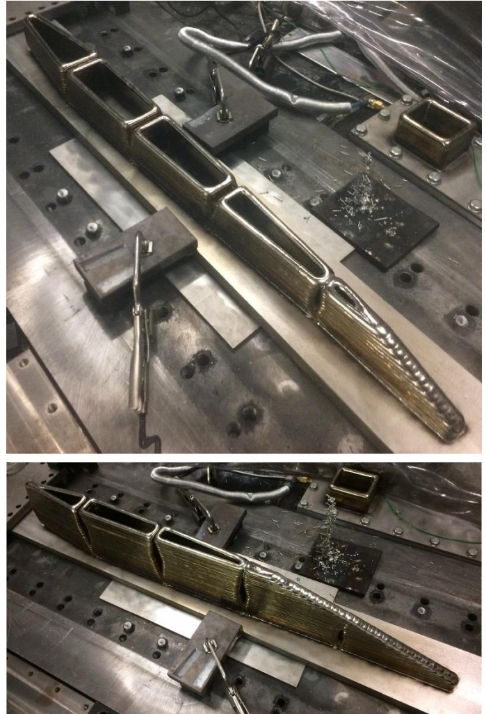
FIGURE 7: PRINTING PROGRESS: LAYER 29 OF 97 (TOP), LAYER 61 OF 97 (BOTTOM)
