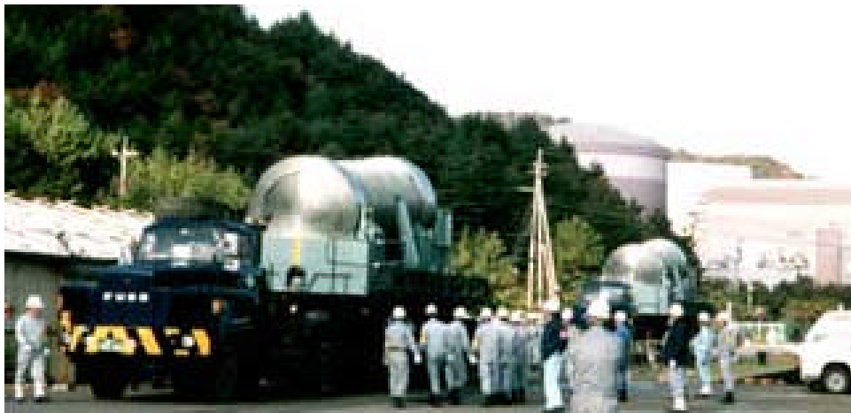
Fig. 2-5. Example of SNF land transport in Japan (Mori 2001).
