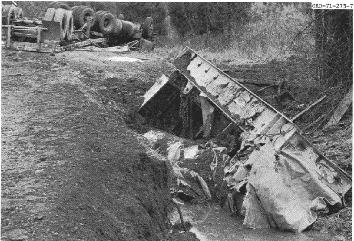
Fig. 4-2. Cask and skid separated from tractor-trailer (Chandler 1972).
