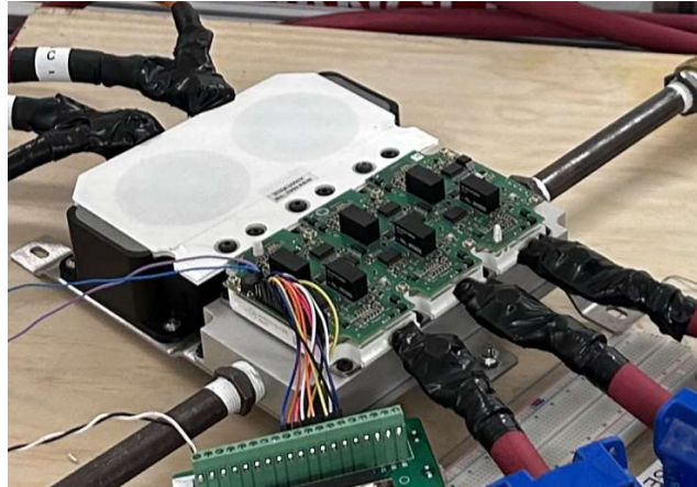
Fig. 5.9. Three-phase stator inverter connected to the prototype.
