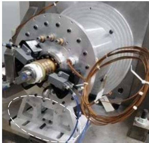
Fig. 5.6. Custom-built support plate attached to the prototype on the test bench.
