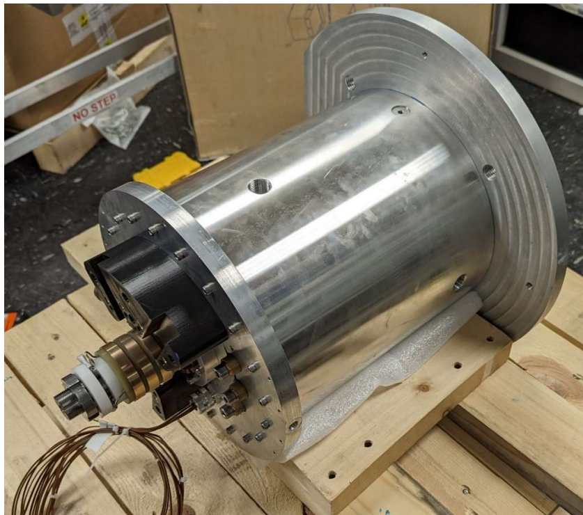
Fig. 2.14. Stator and rotor assembled into the jacket and casing.
