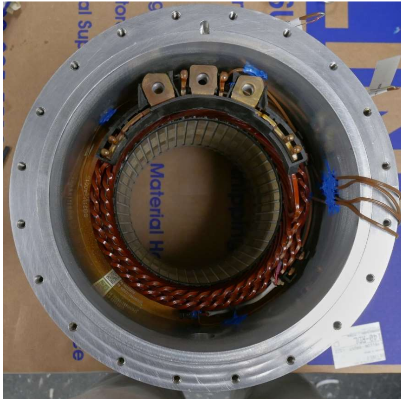
Fig. 2.11. Final assembly of the stator with stator core and jacket.
