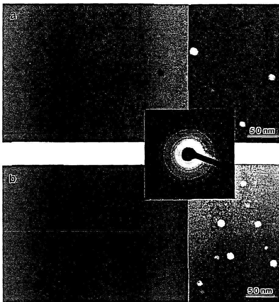
Figure 5: Bright and dark field TEM images of the 150 and 170 keV microstructures which contain FCC particles with an average diameter of 12-13 nm.
