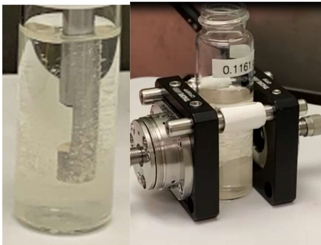
Figure 16: Direct extraction of holmium oxide being monitored using an in-situ dip probe (left) and single pass transmission (right).
