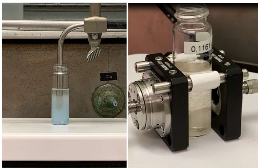
Figure 1: The in-situ dip probe monitoring neodymium oxide (left) and single pass transmission monitoring holmium oxide (right) in an organic solution.
