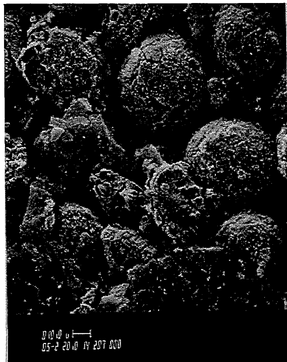
Fig. 45. SEM picture of Ni-coated R02 alloy in particle size 63-90 \mu\text{m} in diameter after 742 cycles.
