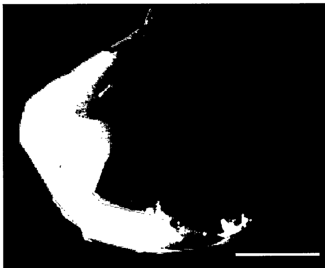
Figure 1. Secondary electron image of a monazite crystal grown in the piston cylinder apparatus at 5 kbar and 600°C (scale bar = 100 \mu\text{m} ). The well-developed crystal faces provide excellent surfaces for the subsequent diffusion anneal. Note that the grayish quench material adhering to the crystal faces is removed prior to the diffusion anneal.
