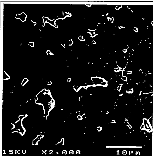
Figure 4: Polished and Thermally Etched Specimen of \text{LaCr}_{0.90}\text{M}_{0.10}\text{O}_3 (1600°C - 6h)
