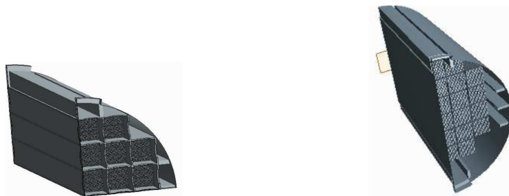
Figure 10. Geometries considered for CFD modeling: previous (left) and current (right).
