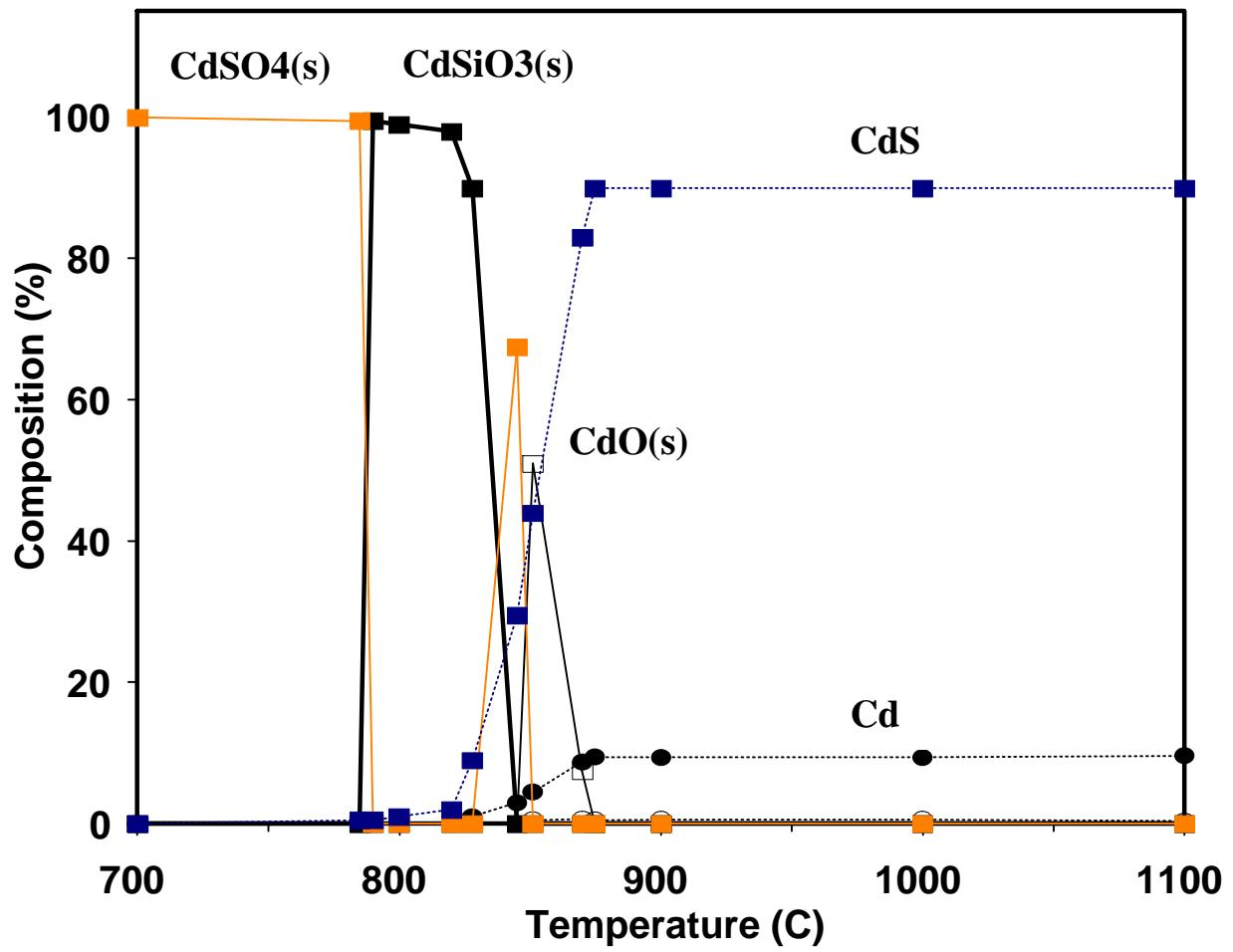
Fig. 3. Simulated cadmium speciation (System: Cd-S-SiO<sub>2</sub>).
