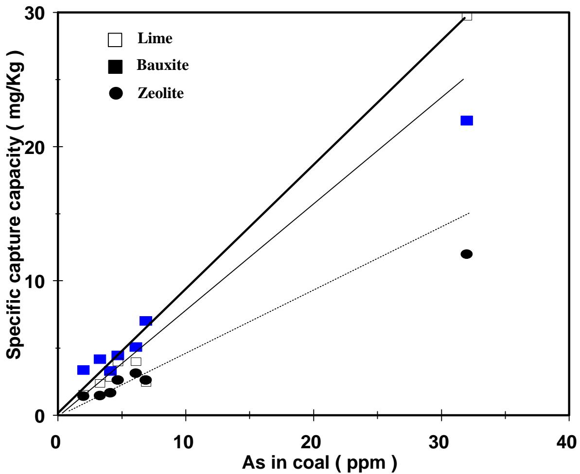
Fig. 7. Specific capture capacity of As by bed sorbents ( $\phi_b$ ).
