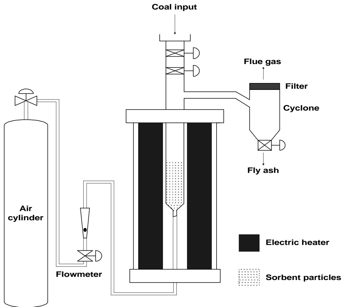
Fig. 1. Fluidized bed coal combustion system.
