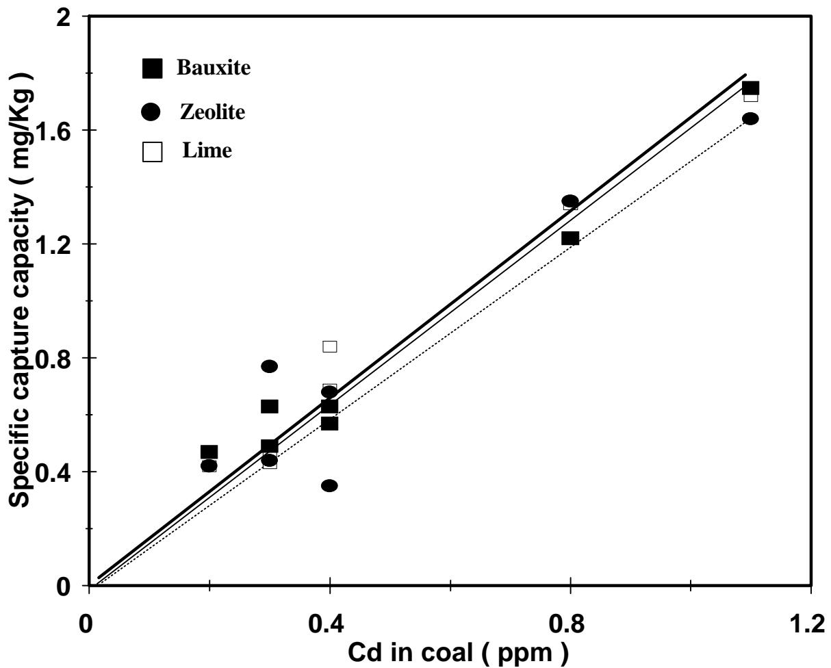
Fig. 6. Specific capture capacity of Cd by bed sorbents ( $\phi_b$ ).
