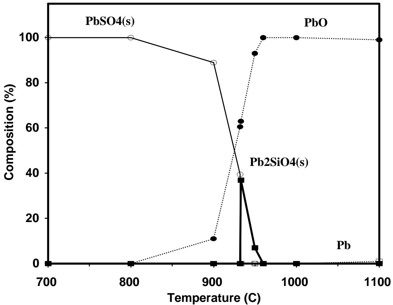
Fig. 2. Simulated lead speciation (System:  $\text{Pb}-\text{S}-\text{SiO}_2$ ).
