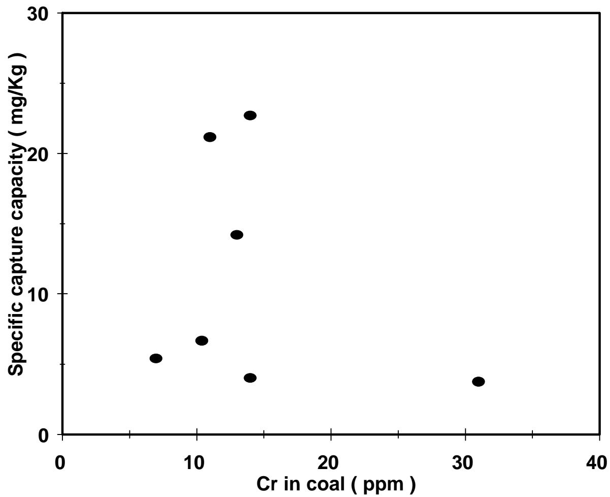
Fig. 8. Specific capture capacity of Cr by Zeolite ( $\phi_b$ ).
