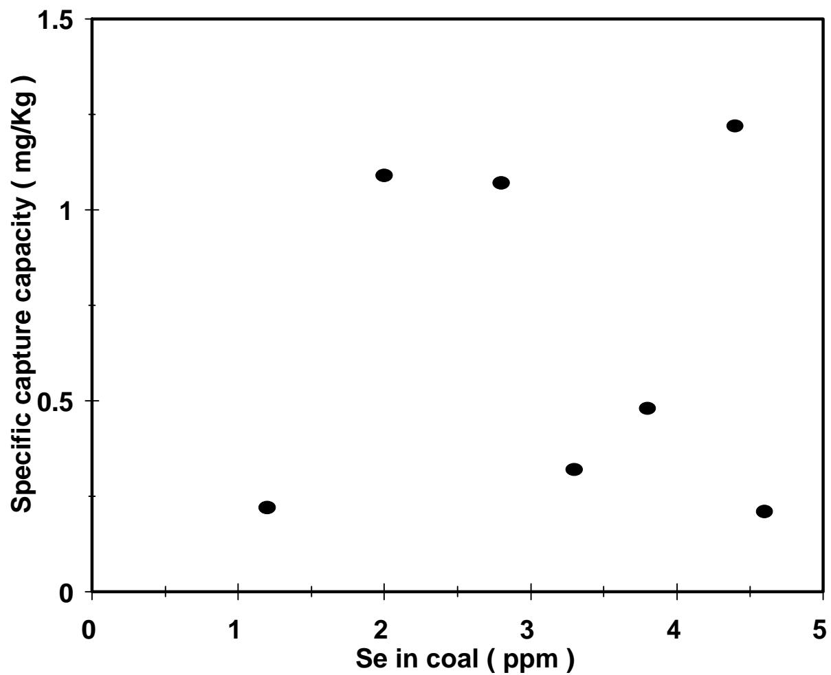
Fig. 9. Specific capture capacity of Se by Zeolite ( $\phi_b$ ).
