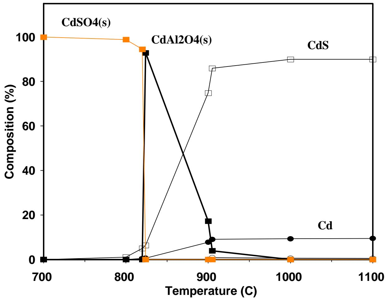
Fig. 4. Simulated cadmium speciation (System: Cd-S-Al<sub>2</sub>O<sub>3</sub>).
