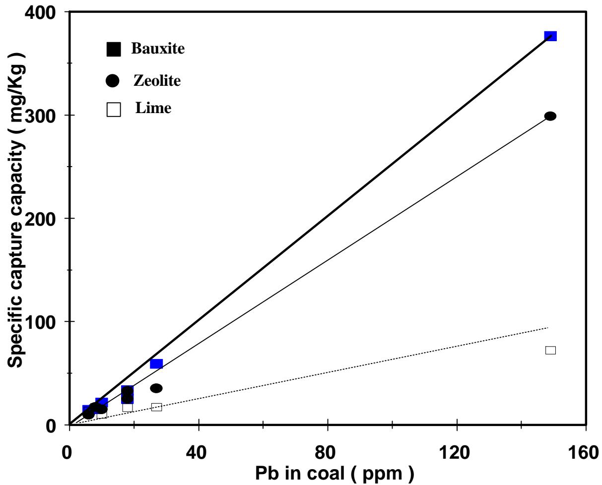
Fig. 5. Specific capture capacity of Pb by bed sorbents ( $\phi_b$ ).
