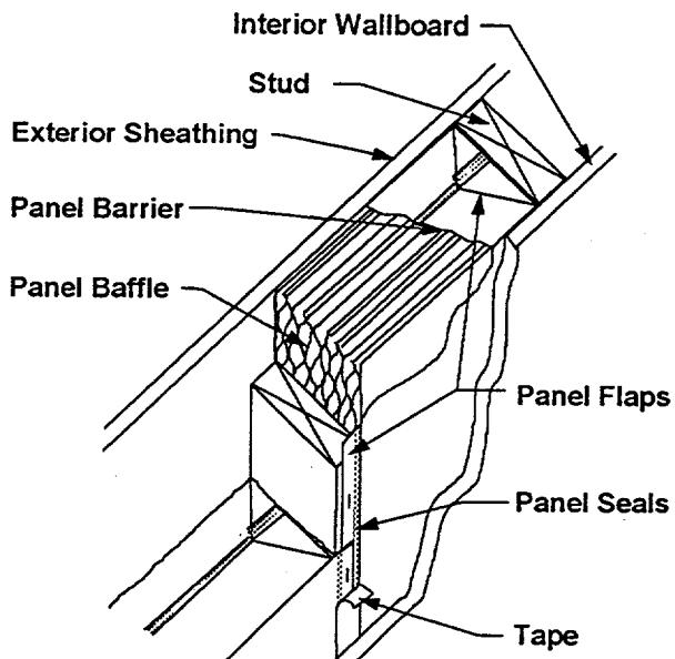
Figure 1. Gas-Filled Panel Installation in Stud Wall
