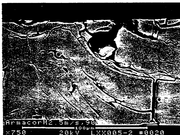
Figure 4 The cross section of arc-sprayed FeCrSiB coating eroded at V=2.5 m/s, \alpha=90^\circ .
