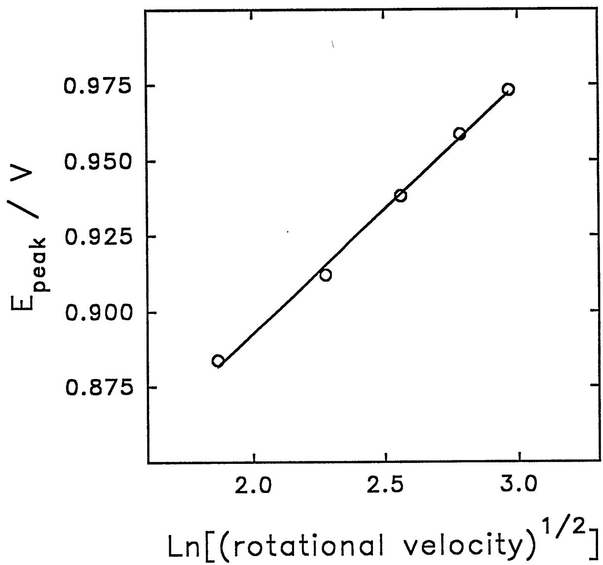
Figure 3.10. Correlation of peak potential for ethylamine with square root of rotational velocity in 1.0 M carbonate buffer (pH 10). Concentration: 2.50 mM.
