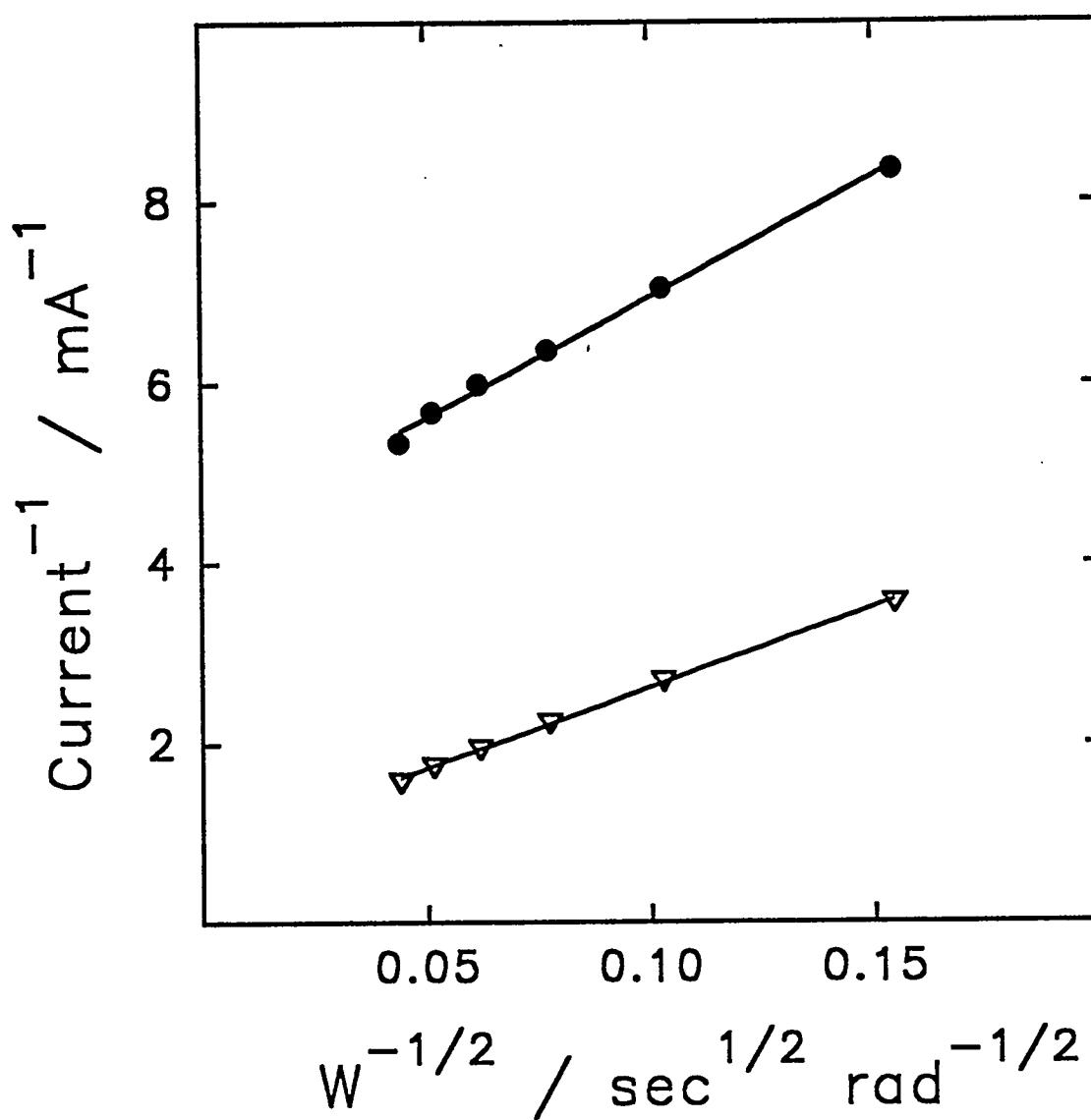
Figure 3.5. Representative Koutecky-Levich plots for 2.00 mM alanine in 1.0 M carbonate buffer (pH 10). Temperature (°C): (●) 10, (▽) 40.
