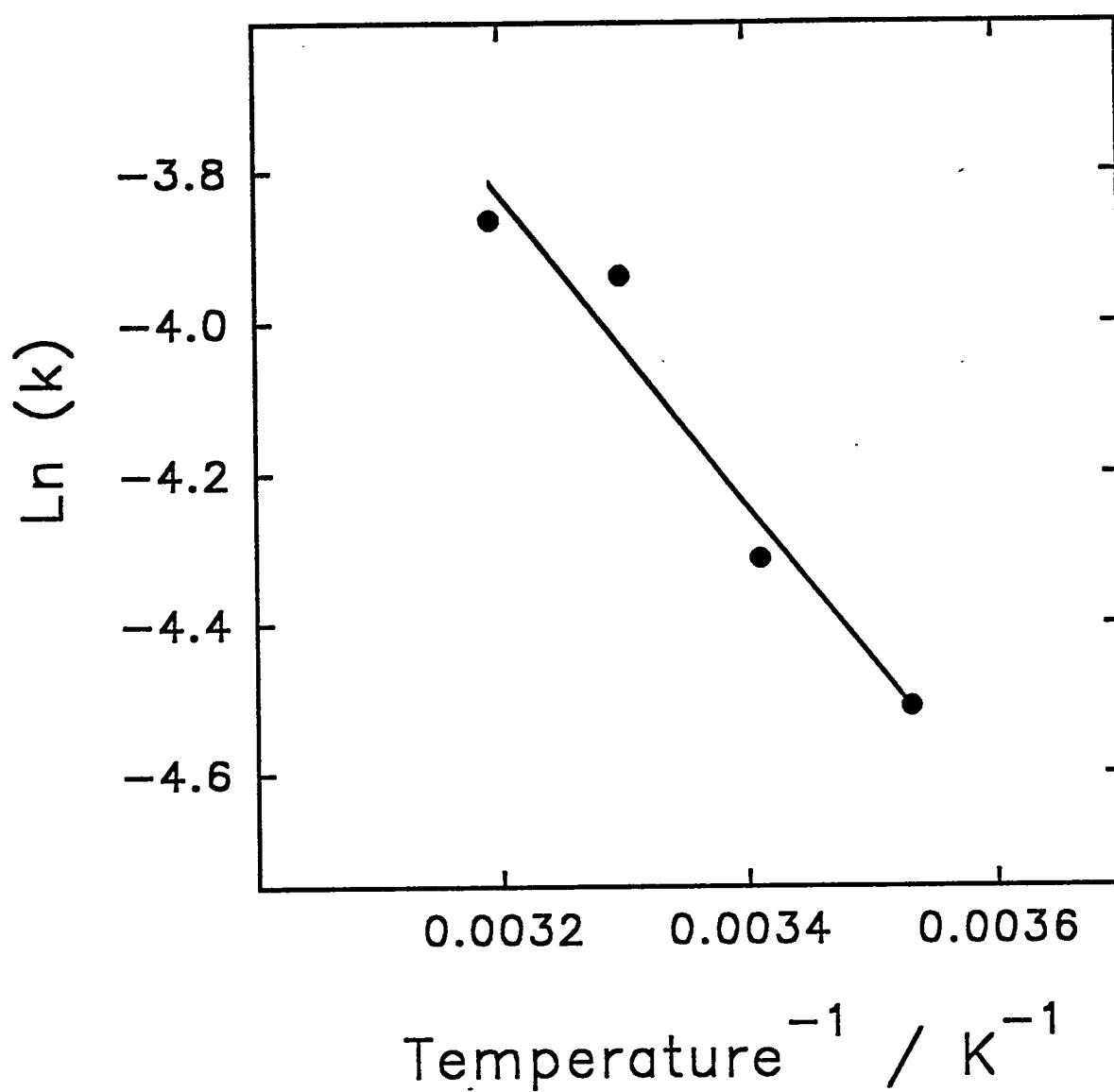
Figure 3.6. Arrhenius plot for 2.56 mM ethylamine in 1.0 M carbonate buffer (pH 10).
