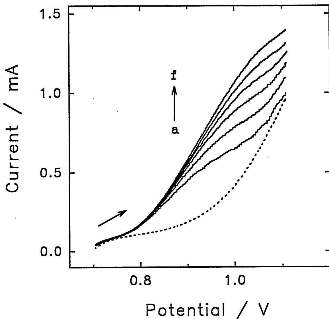
Figure 1.3. Voltammetric response (pos. scan) for ethylamine at an anodized eutectic-phase Ag-Pb alloy RDE as a function of rotation speed in 0.1 M carbonate buffer (pH 10). Scan rate: 2.0 V min<sup>-1</sup>. Ethylamine concentration (mM): (---) 0, (—) 2.0. Rotation speed (rev min<sup>-1</sup>): (a) 400, (b) 900, (c) 1600, (d) 2500, (e) 3600, (f) 4900.
