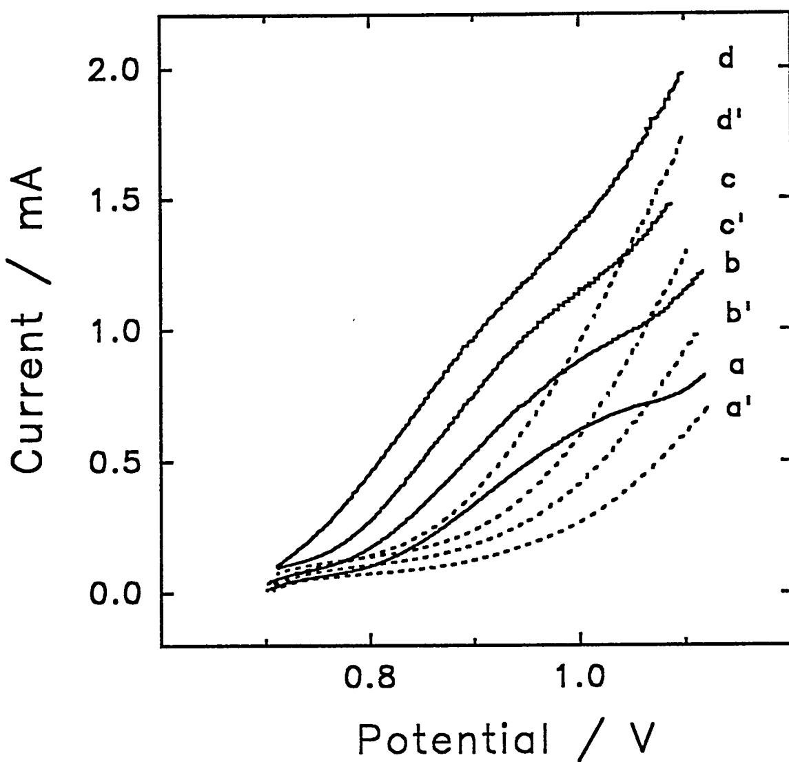
Figure 3.3. Voltammetric response for 2.0 mM ethylamine as a function of temperature in 1.0 M carbonate buffer (pH 10). Scan rate: 2.0 V min<sup>-1</sup>. Rotation: 168 rad s<sup>-1</sup>. Curves: (---) residual, (—) ethylamine. Temperature (°C): (a,a') 10, (b,b') 20, (c,c') 30, (d,d') 40.
