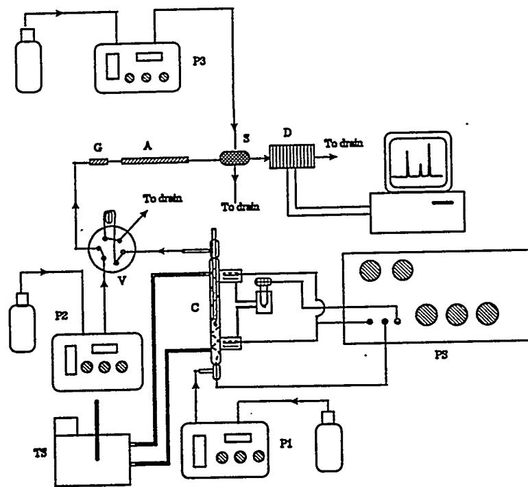
Figure 3.2. Schematic diagram of the interface between the flow-through reactor and the Ion Chromatography. Components: (P1) pump-1, (P2) pump-2, (P3) pump-3, (C) flow-through reactor, (TS) thermostat, (V) valve, (G) guard column, (A) analytical column, (S) suppressor, (D) conductivity detector.
