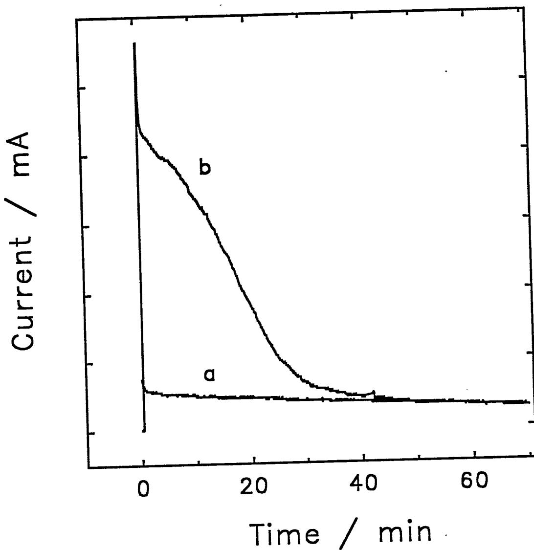
Figure 2.5. Current-time profiles for the exhaustive electrolysis of ethylamine in stirred 0.1 M carbonate buffer (pH 10). Wire electrode (ca.  $9\text{ cm}^2$ ): anodized eutectic phase of Ag-Pb alloy. Potential: 1.0 V vs. SCE. Curves: (a) residual, (b) 17.5 mM  $(\text{NH}_4)_2\text{SO}_4$ .
