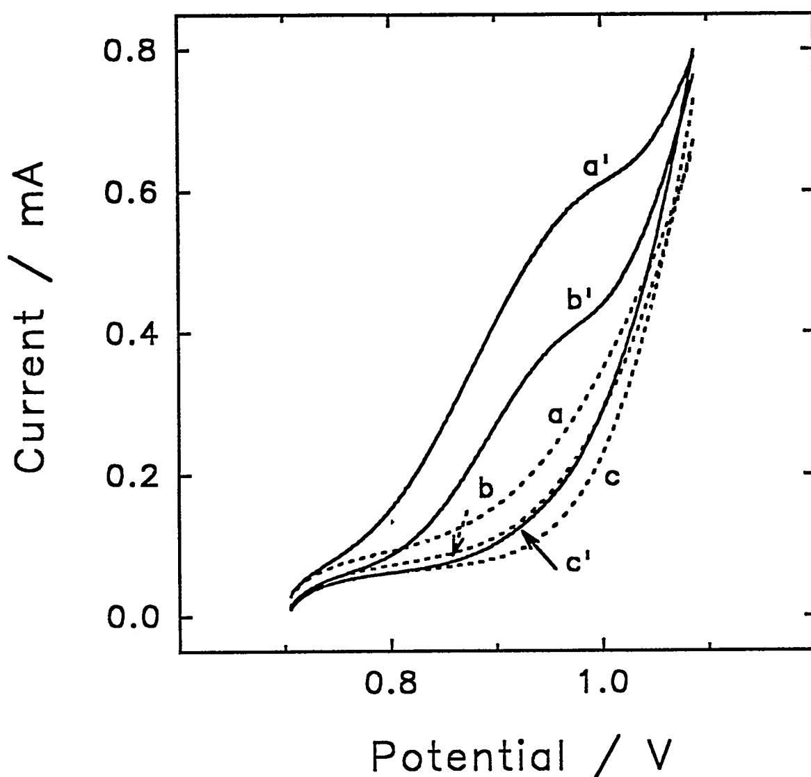
Figure 1.4. Effect of added  $\text{Cl}^-$  on voltammetric response (pos. scan) for ethylamine at an anodized eutectic-phase Ag-Pb RDE in 0.1 M carbonate buffer (pH 10). Scan rate:  $2.0 \text{ V min}^{-1}$ . Rotation speed:  $1600 \text{ rev min}^{-1}$ . Curves: (---) residual, (—) 2.0 ethylamine. Concentration  $\text{NaCl}$  (mM): (a,a') 0, (b,b') 10, (c,c') 100.
