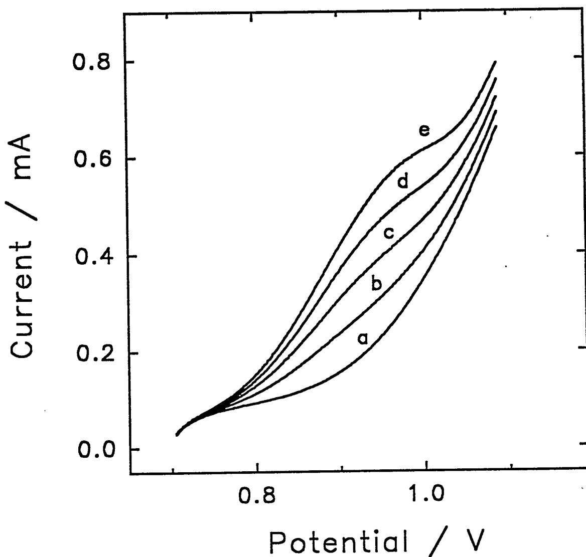
Figure 1.2. Voltammetric response (pos. scan) at an anodized eutectic-phase Ag-Pb alloy RDE as a function of ethylamine concentration in carbonate buffer (pH 10). Scan rate:  $2.0 \text{ V min}^{-1}$ . Rotation speed:  $1600 \text{ rev min}^{-1}$ . Ethylamine concentration (mM): (a) 0, (b) 0.5, (c) 1.0, (d) 1.5, (e) 2.0.
