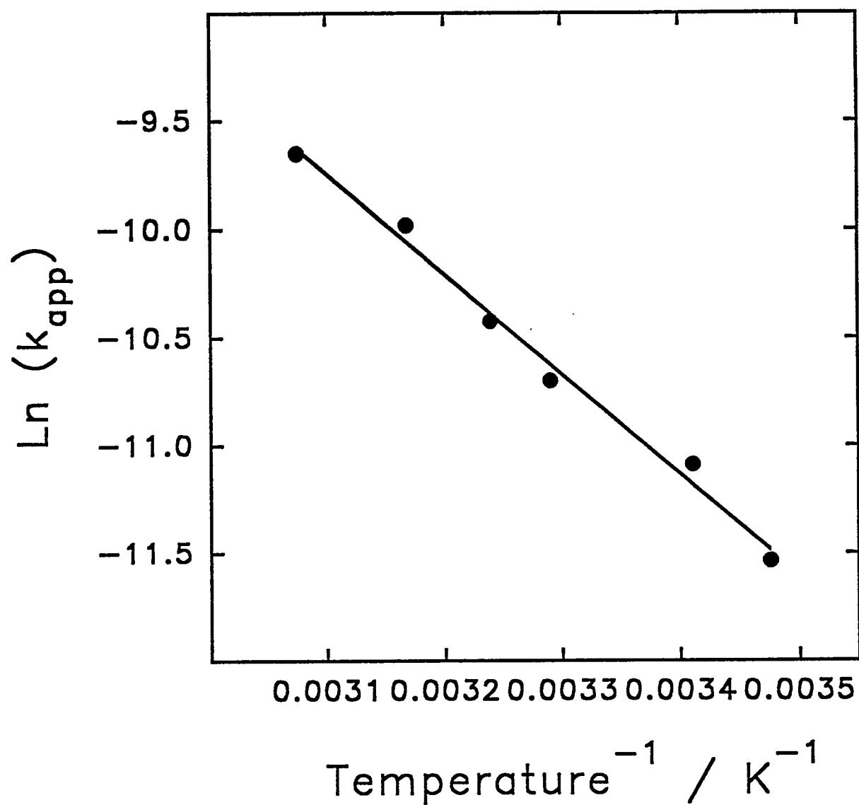
Figure 3.9. Arrhenius plot for oxidation of  $NH_3(aq)$  in flow-through reactor.
