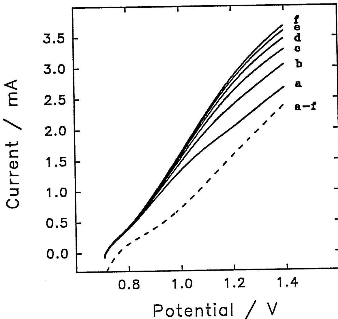
Figure 2.1. Voltammetric responses (pos. scan) for  $(\text{NH}_4)_2\text{SO}_4$  at an anodized eutectic-phase Ag-Pb alloy disk electrode as a function of rotation speed in 0.1 M carbonate buffer (pH 10). Scan rate: 2.0 V  $\text{min}^{-1}$ . Concentration of  $(\text{NH}_4)_2\text{SO}_4$  (mM): (---) 0, (—) 1.0. Rotational velocity ( $\text{rad s}^{-1}$ ): (a) 42, (b) 94, (c) 168, (d) 262, (e) 377, (f) 513.
