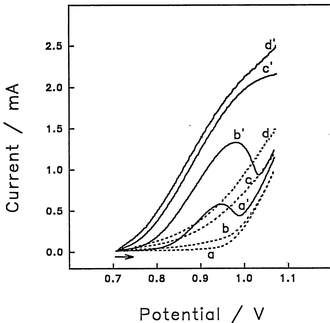
Figure 1.1. Voltammetric response (pos. scan) for ethylamine at various electrodeposited Ag-Pb oxide rotated disk electrodes in carbonate buffer (pH 10). Scan rate: 2.0 V min<sup>-1</sup>. Rotation speed: 3600 rev min<sup>-1</sup>. Film-deposition solution: 40  $\mu$ M Pb(II) with variable Ag(I) in carbonate buffer (pH 10); [Ag(I)]/[Pb(II)]: (a,a') 1/40, (b,b') 1/10, (c,c') 1/4, (d,d') 1/2. Ethylamine concentration (mM): (----) 0, (—) 3.9.
