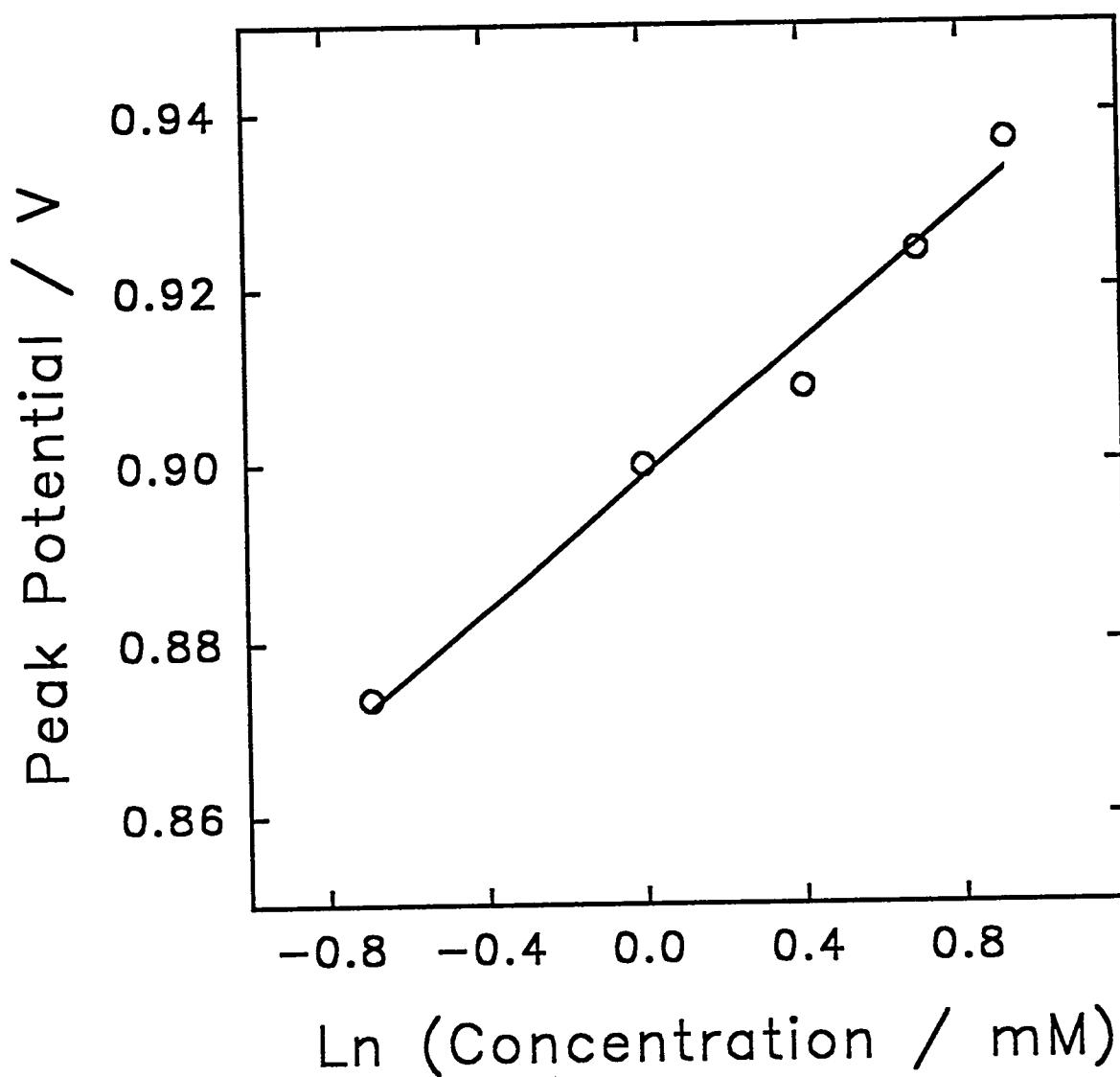
Figure 3.11. Correlation of peak potential for ethylene as a function of concentration in 1.0 M carbonate buffer (pH 10). Rotation: 168 rad s<sup>-1</sup>.
