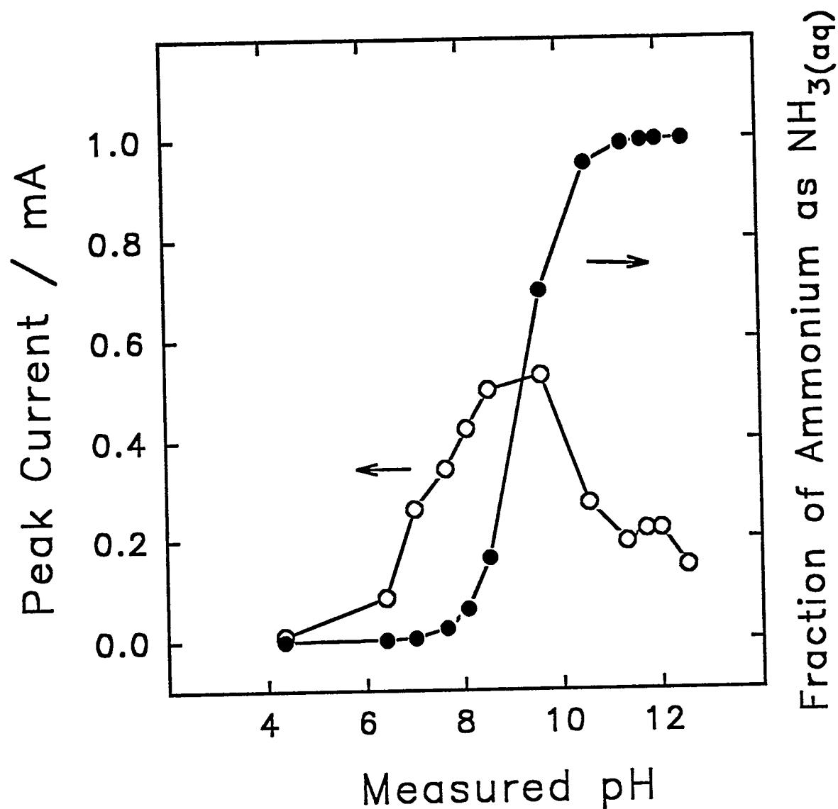
Figure 2.3. Correlation of voltammetric peak response and calculated concentration of  $\text{NH}_3\text{(aq)}$  as a function of pH. Buffer: 50 mM  $\text{NaH}_2\text{PO}_4$  adjusted to pH by NaOH. Scan rate: 2.0 V  $\text{min}^{-1}$ . Rotational velocity: 168 rad  $\text{s}^{-1}$ .
