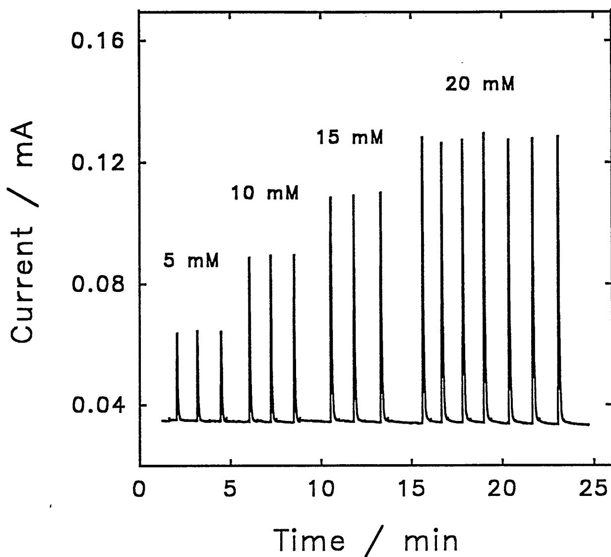
Figure 1.5. Representative flow-injection detection peaks for ethylamine at an anodized eutectic-phase Ag-Pb alloy electrode in 0.1 M carbonate buffer (pH 10). Carrier phase: 0.1 M carbonate buffer,  $1.0 \text{ mL min}^{-1}$ . Potential: 0.90 V vs. SCE. Sample loop:  $50 \mu\text{L}$ . Ethylamine concentrations: given in figure.
