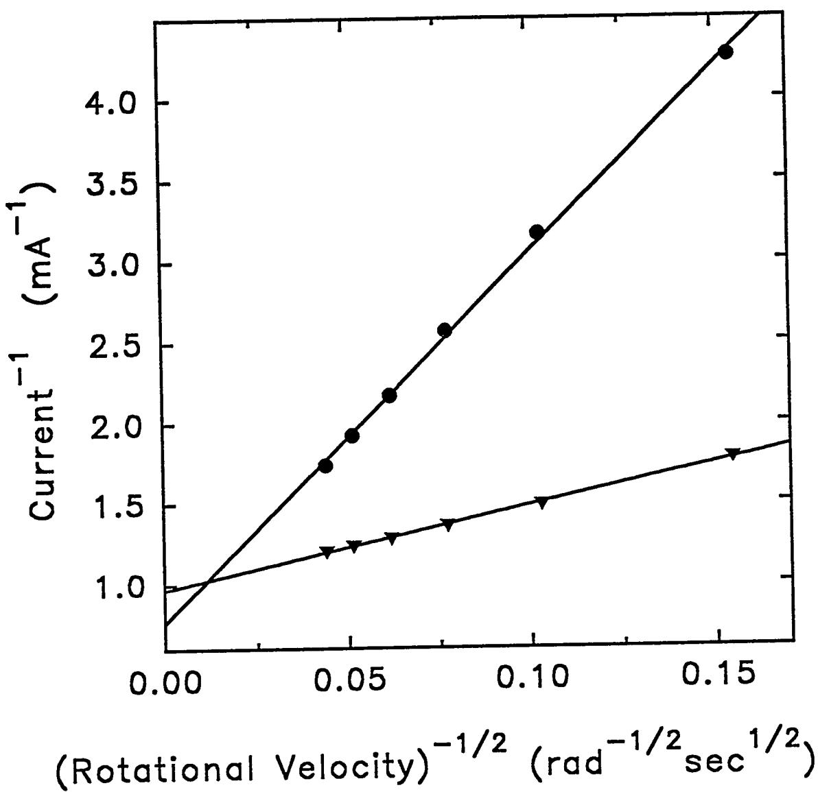
Figure 2.2. Koutecky-Levich plots for voltammetric peak responses for ( $\nabla$ ) 2.0 mM  $\text{NH}_4\text{HCO}_3$  and ( $\bullet$ ) 2.0 mM ethylamine in 0.1 M carbonate buffer (pH 10). Scan rate: 2.0 V min<sup>-1</sup>.
