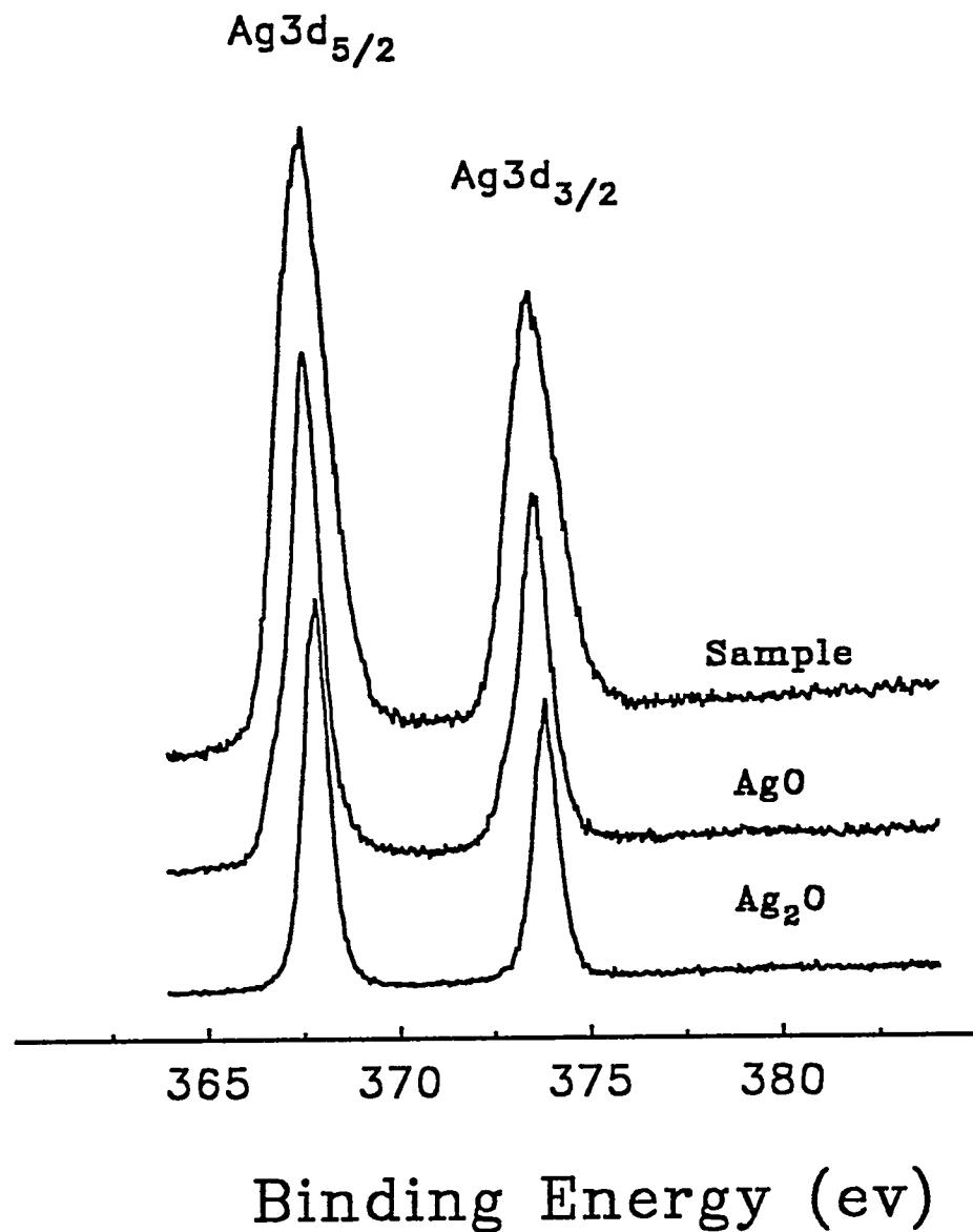
Figure 1.7. X-ray photon spectra showing  $\text{Ag 3d}_{5/2}$  peaks for specified samples.
