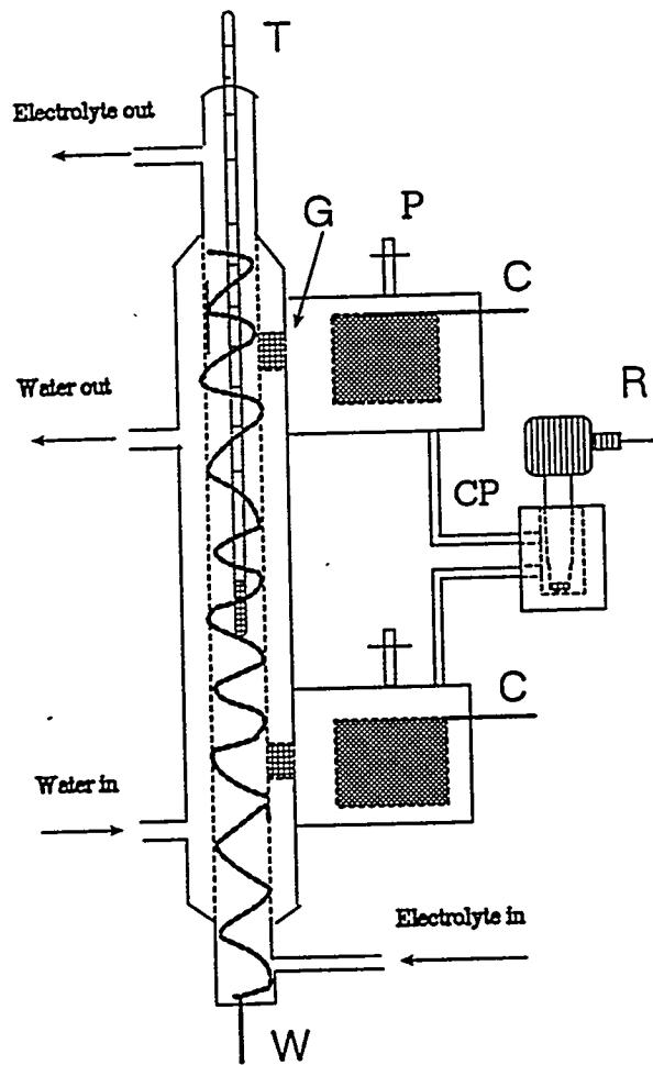
Figure 3.1. Schematic diagram of water-jacketed flow-through electrolysis reactor. Components: (C) counter electrodes, (G) fritted glass disks, (R) reference electrode, (W) working electrode, (CP) capillary tube, (P) pressure valve, (T) thermometer.
