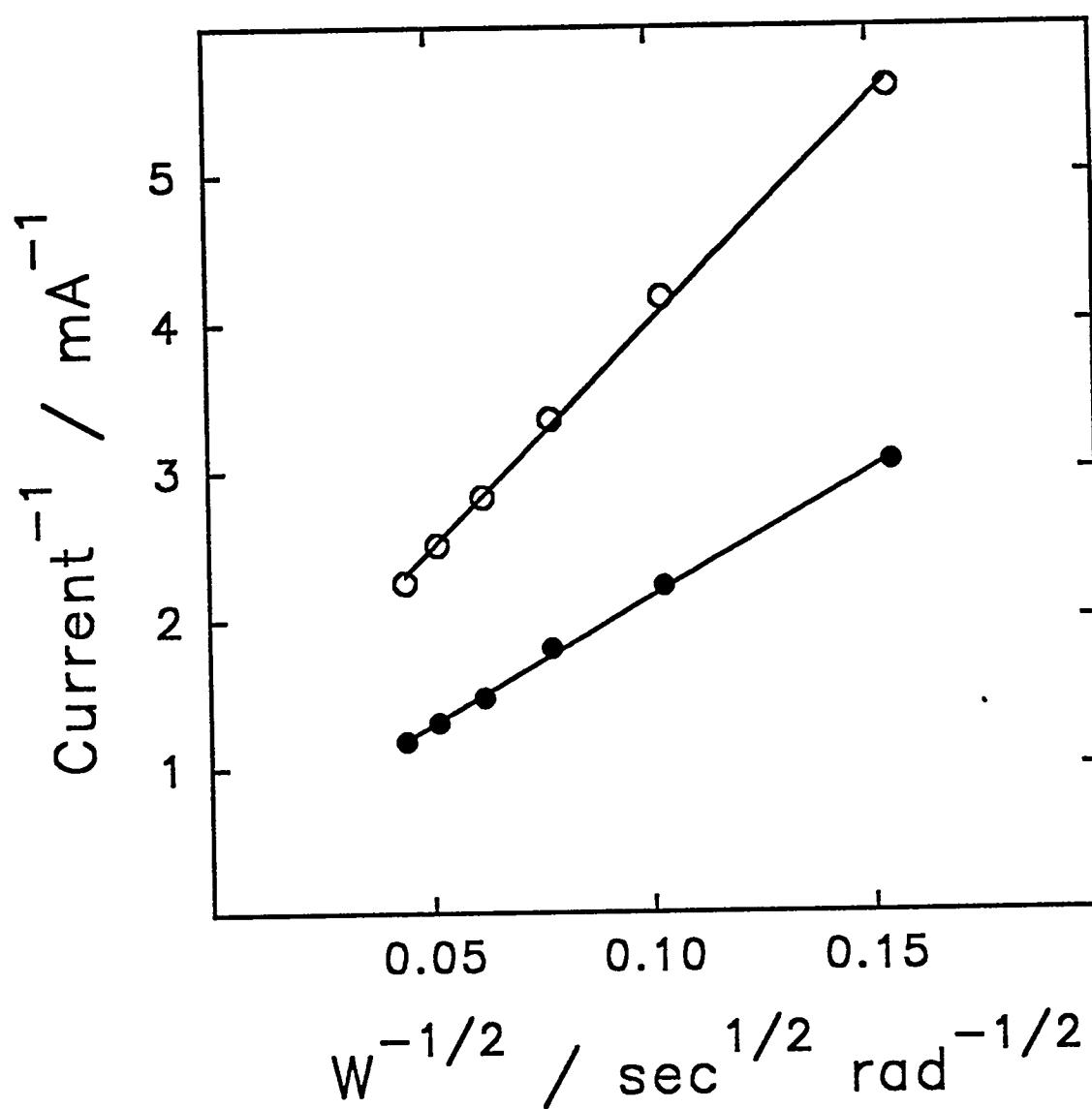
Figure 3.4. Representative Koutecky-Levich plots for 2.56 mM ethylamine in 1.0 M carbonate buffer (pH 10). Temperature (°C): (○) 10, (●) 40.
