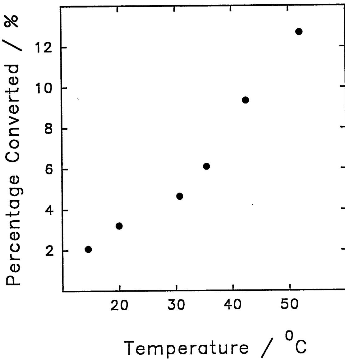
Figure 3.8. Percent conversion of total ammonia to nitrate ion in the flow-through reactor as a function of temperature. Flow rate:  $8.2 \times 10^{-3} \text{ cm}^3 \text{ s}^{-1}$  (0.50 mL  $\text{min}^{-1}$ ).
