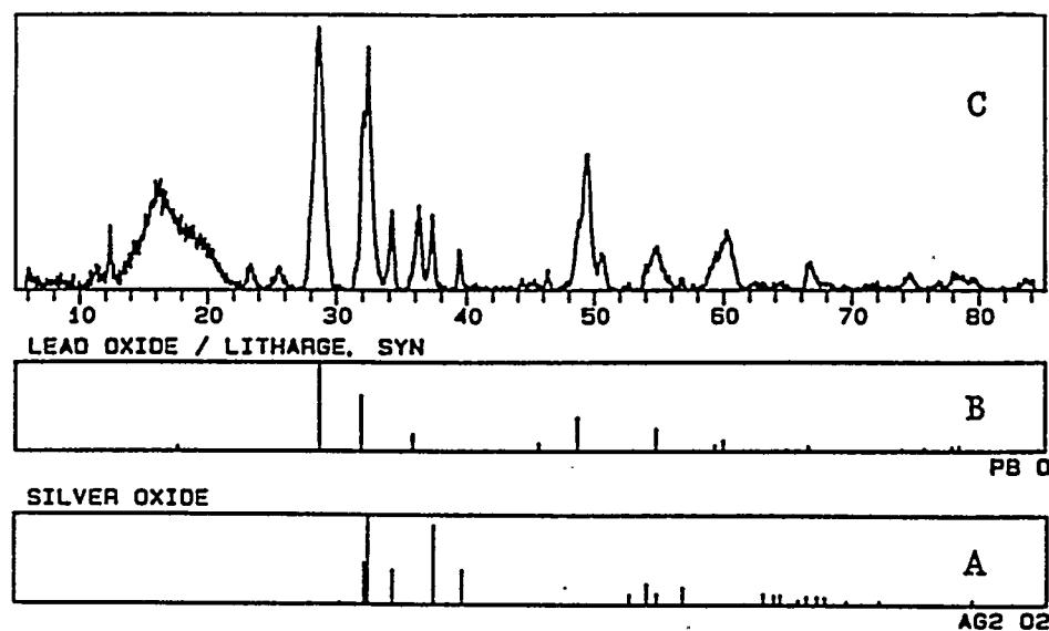
Figure 1.6. X-ray diffraction spectra: (A) silver oxide ( $\text{AgO}$ ); (B) litharge ( $\text{PbO}$ ); and (C) surface of 1:5 (wt:wt) Ag-Pb alloy electrode anodized in 0.1 M carbonate buffer (pH 10) at 0.90 V for 12 hrs.
