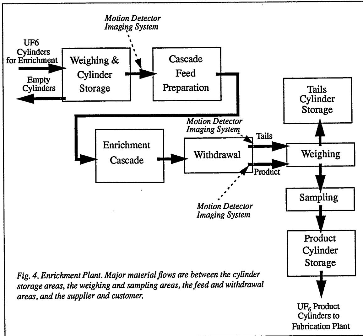
*Fig. 4. Enrichment Plant. Major material flows are between the cylinder storage areas, the weighing and sampling areas, the feed and withdrawal areas, and the supplier and customer.*
