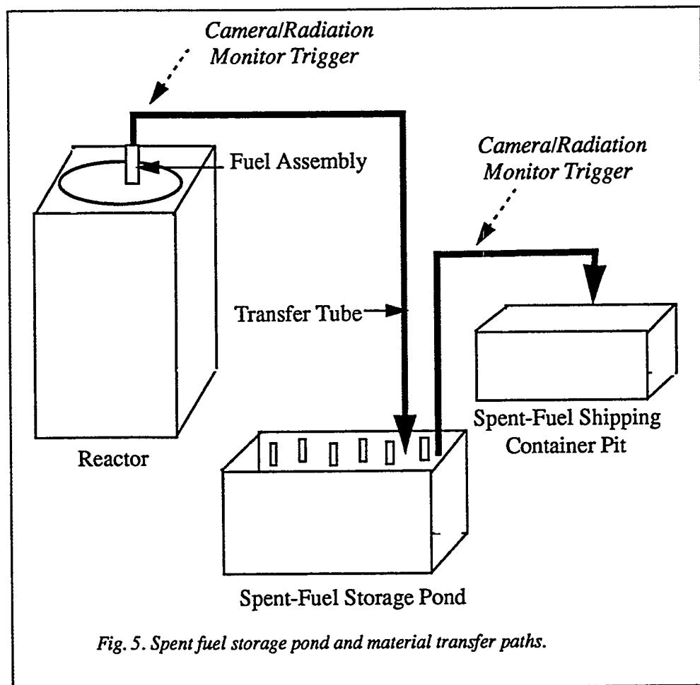
*Fig. 5. Spent fuel storage pond and material transfer paths.*
