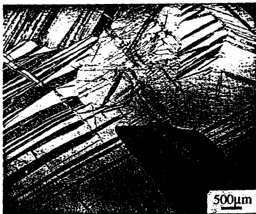
Fig. 1. Optical micrograph showing deformation products of \text{Ti-34mol.\%Al} deformed in compression to about 8% strain at 1273K.
