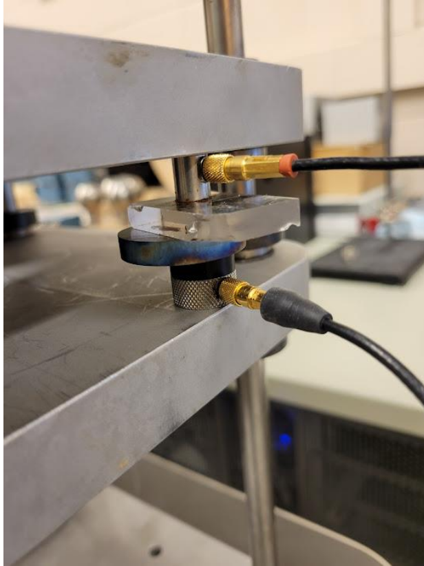
Figure 2.7. Sample coupled to fused quartz and shear transducers with reference for Method 2 time measurement.
