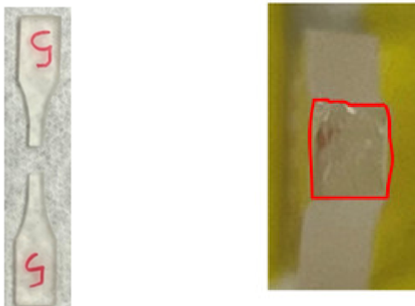
Figure 20. Tension samples post-tension tests and cross-section (right)
