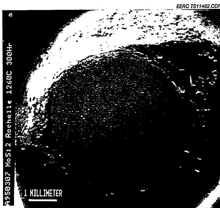
Figure 2. SEM photo showing a decrease in thickness of the MoSi 2 and reaction at the slag-MoSi 2 interface.
