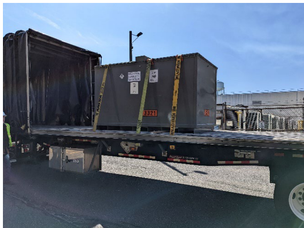
Figure 5-8 Truck with B-box for shipping LLW to NNSS
