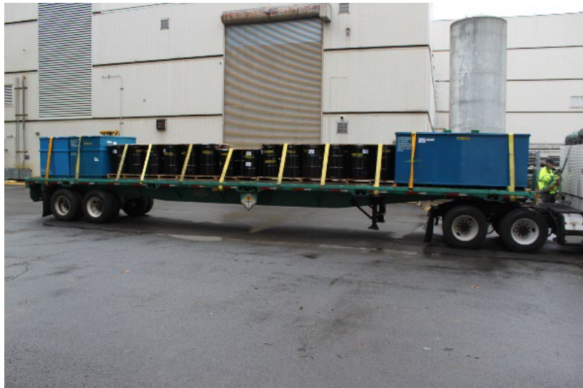
Exhibit 5-7. Truck with B-boxes and drums for shipping LLW to Energy Solutions
