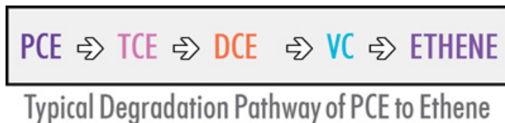
Exhibit 6-7. Typical PCE Degradation Pathway
