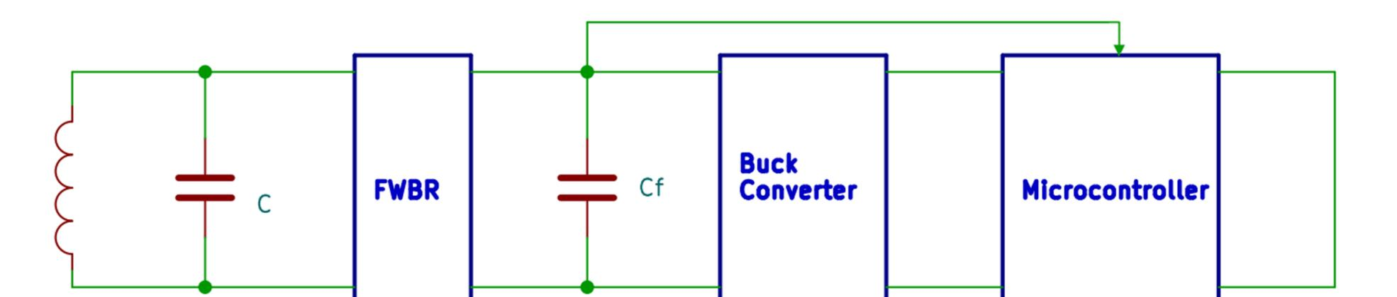
Fig. 2. Circuit for the Sensor Nodes
