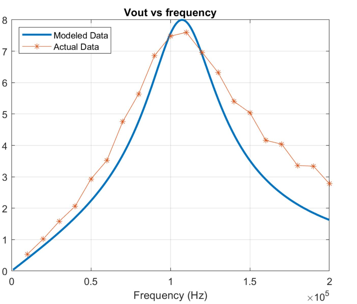
Fig. 5. Modeling Results for Parallel-Resonant Coupling for 150Ω load
