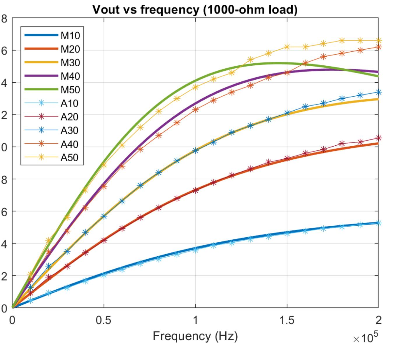
Fig. 4. Modeling Results for Inductive Coupling using 1kΩ load
