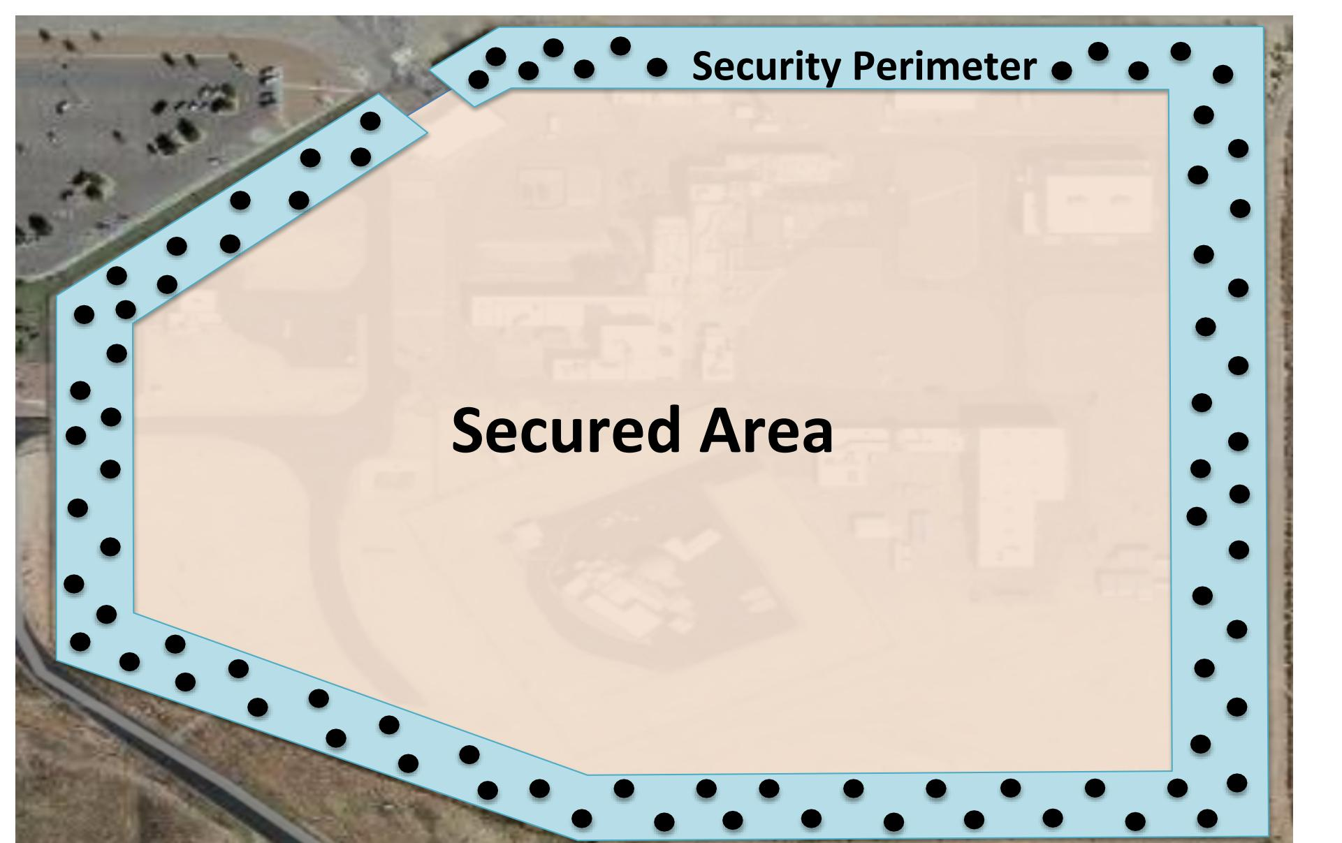
Fig. 3. Security Perimeter with Wireless Sensor Nodes
