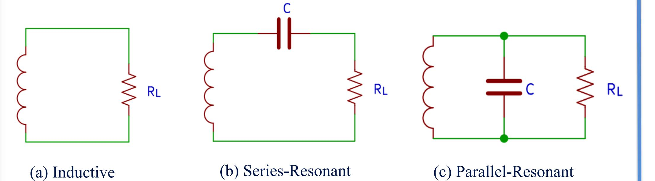
Fig. 1. Configurations for the Transmit Loop & Receiver Nodes
