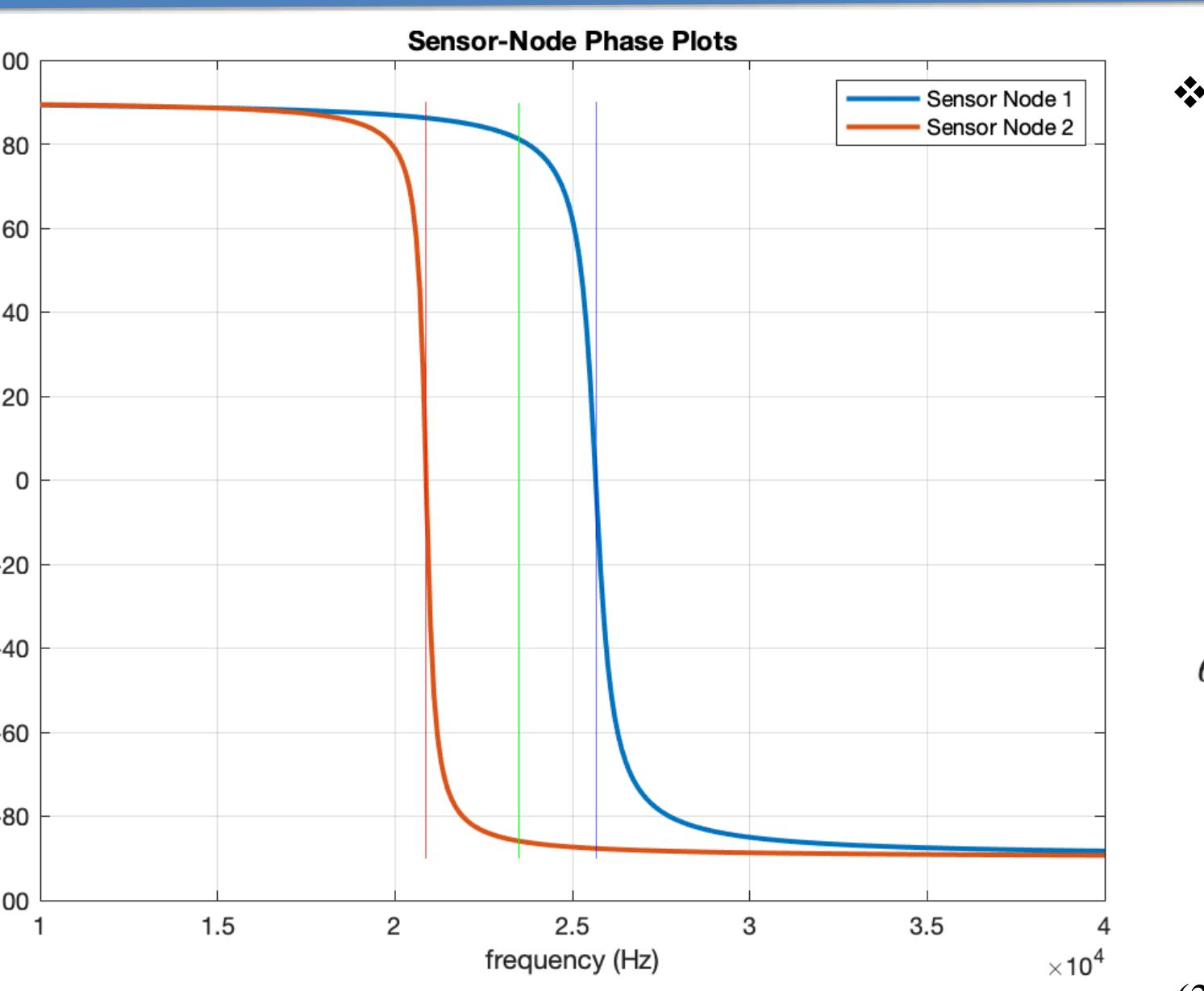
Fig. 6. Condition for Additive Coupling Between Sensor Nodes
