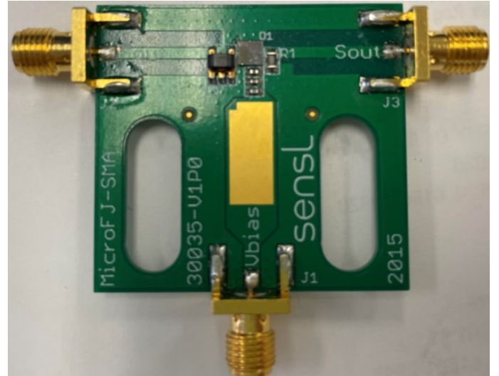
Fig. 6: MicroFJ SiPM mounted on evaluation board.
