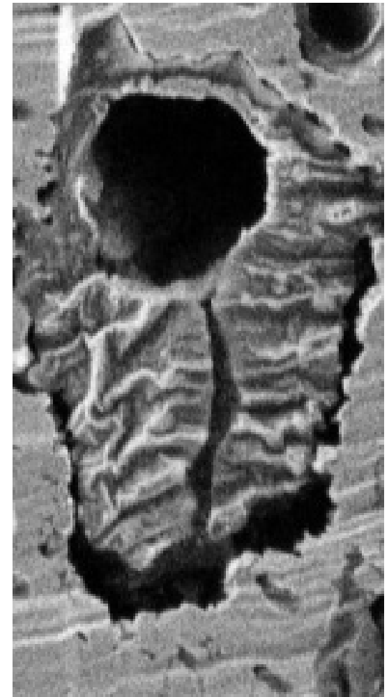
Bitumen-extracted shale with collapsed kerogen
