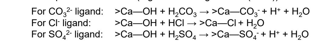
Total consolidation of granular calcite depend on the aqueous ligand present in solution (Figure 1b from Choens et al. (2021)).
