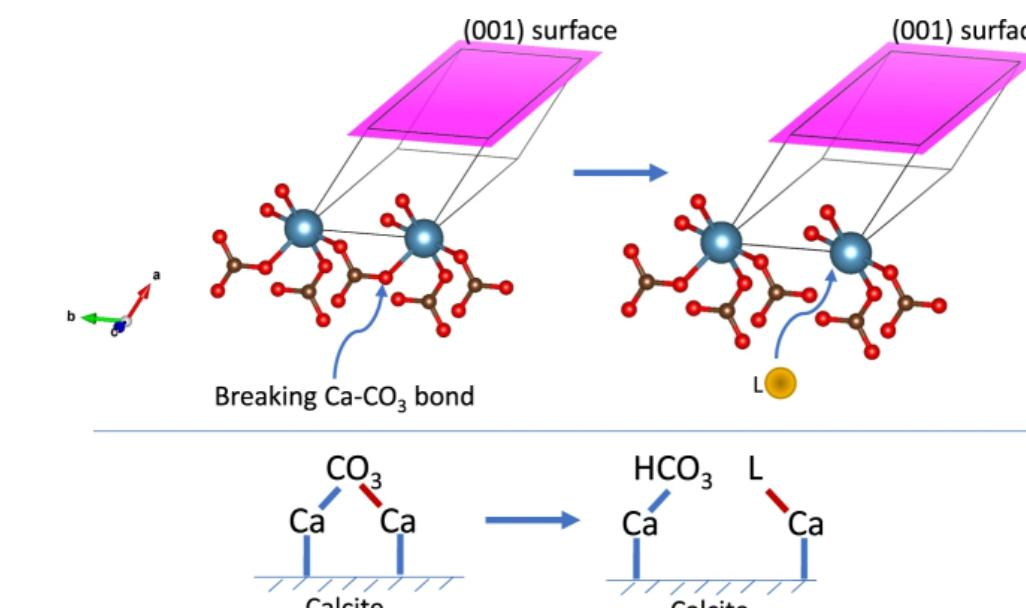
The conceptual model for chemical interaction at the crack tip shows subcritical fracturing is controlled by the chemical ligand's, L, ability to form complexes with calcite (Figure 7 from Ilgen et al. (2018)).
