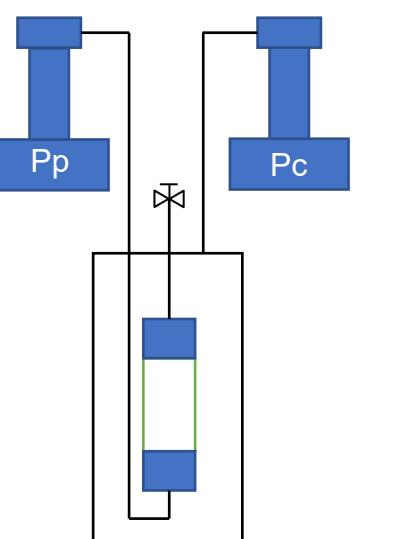
Consolidation setup: Independent confining and pore pressure syringe pumps. Pore fluid was flowed from bottom to top of sample under a small confining pressure and valved closed during testing for single ended drainage.
