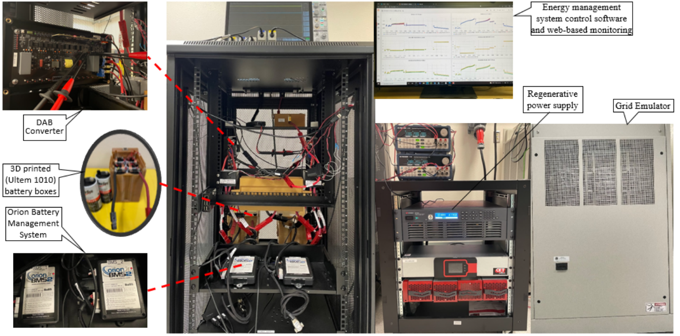
Fig. 3. Hardware setup developed for testing hybrid battery system that consists of Lithium-iron-phosphate and Lead-acid battery packs.
