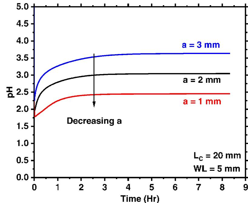
For atmospheric exposures, larger  $a$  increases  $i_{c,loc}$ , limits  $[\text{MCl}_x]$ , and allows high pH
