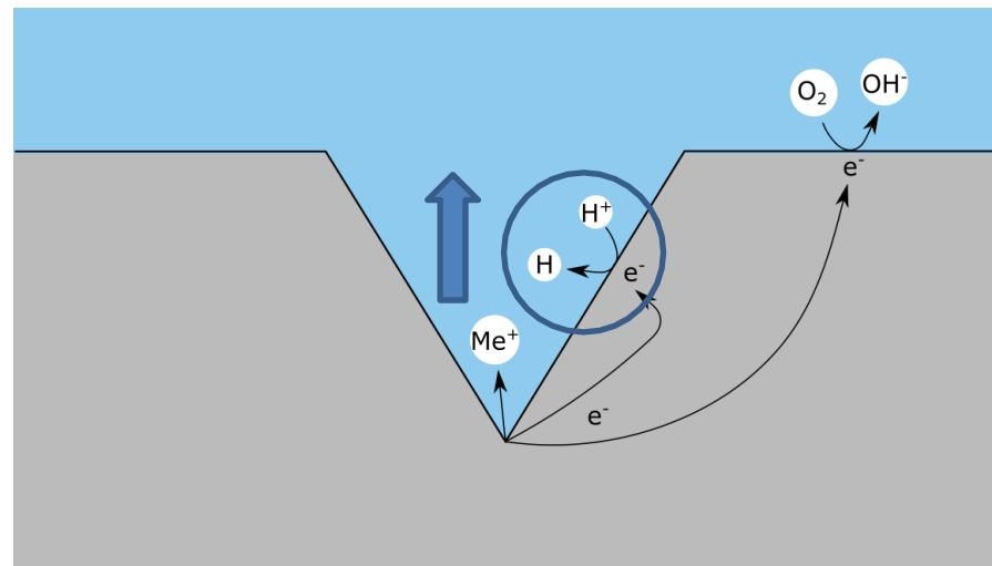
$$\text{Fraction of Cathodic Current} = \frac{i_{cathodic}}{i_{anodic}}$$
