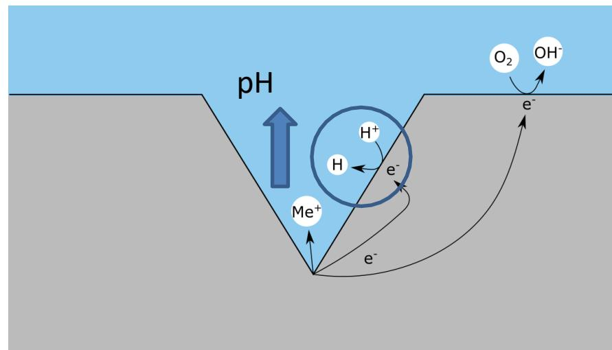
$$\text{Fraction of Local Cathodic Current} = \frac{i_{cathodic}}{i_{anodic}}$$
