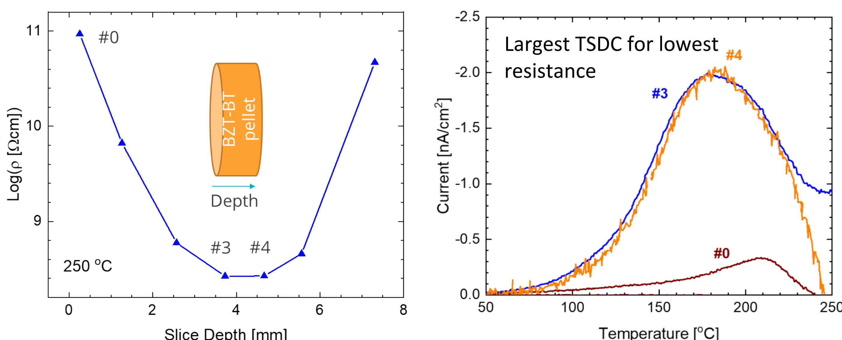
Polarization temperature dependence and mechanism of TSDC
