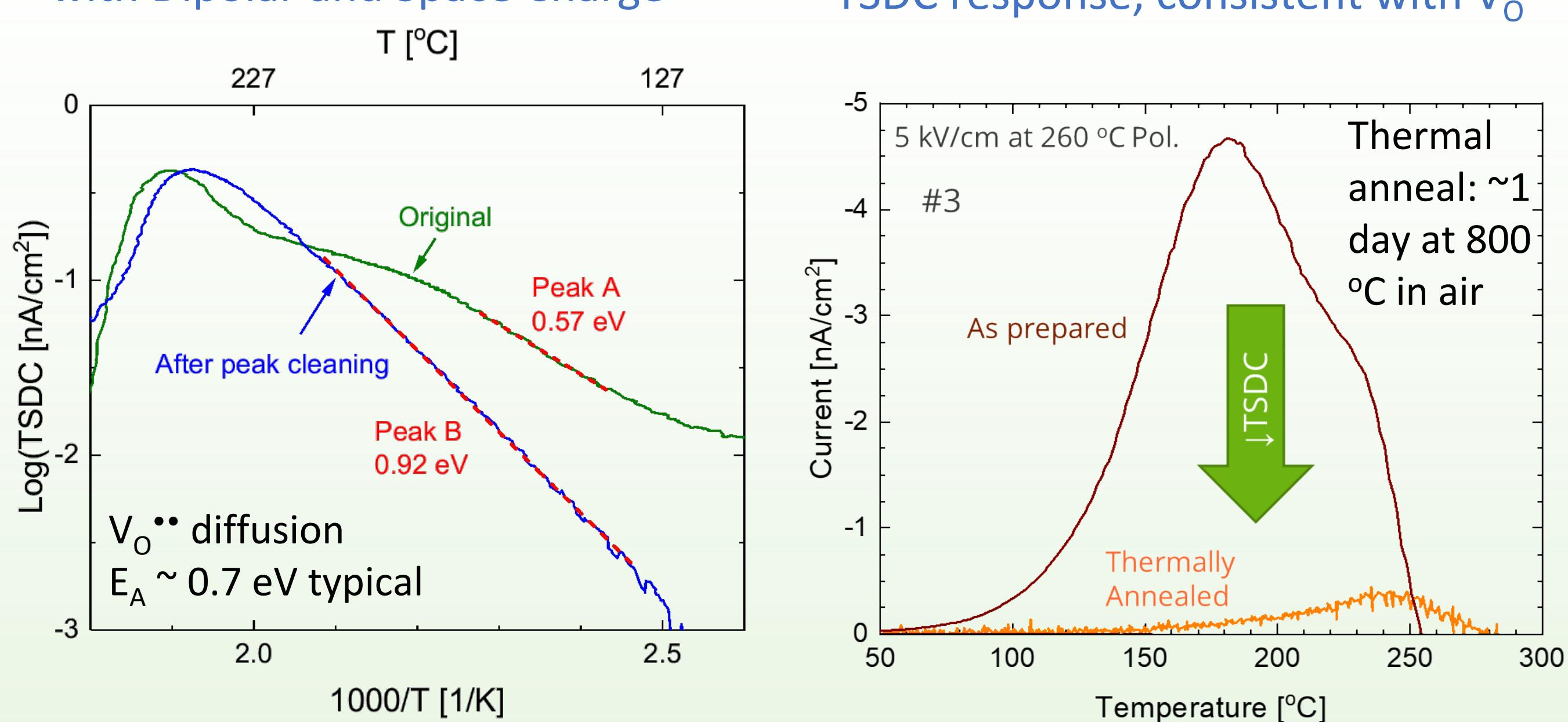
DC lifetime increased with thermal annealing
