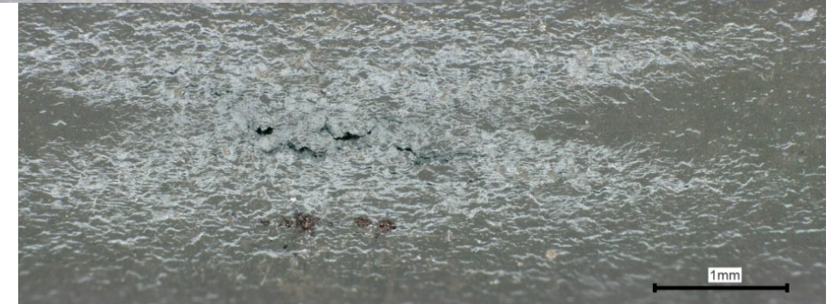
Below: Example crack in 316 tube (tested at 4750 psi)
