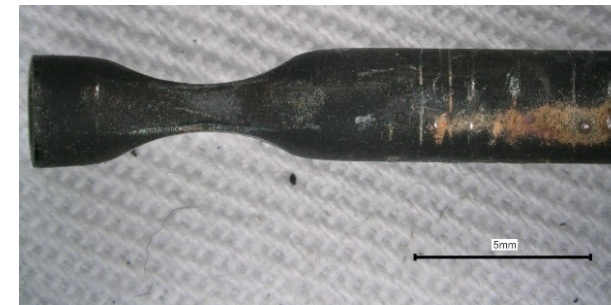
Left: 316 pinch weld showing notable oxidation
