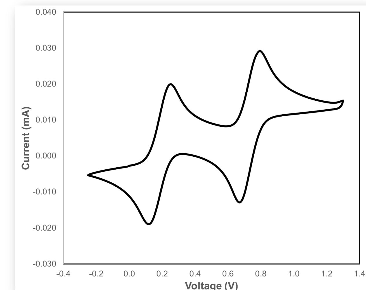
Using cyclic voltammetry, we determined molecular oxygen could oxidize this complex.
