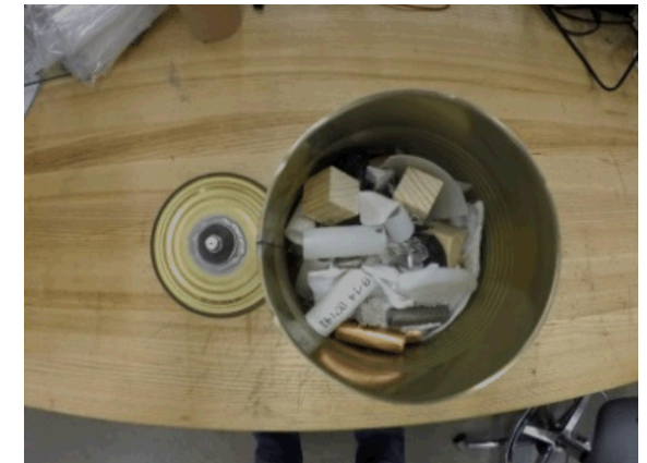
1/4-Scale Drum (with surrogate waste)
