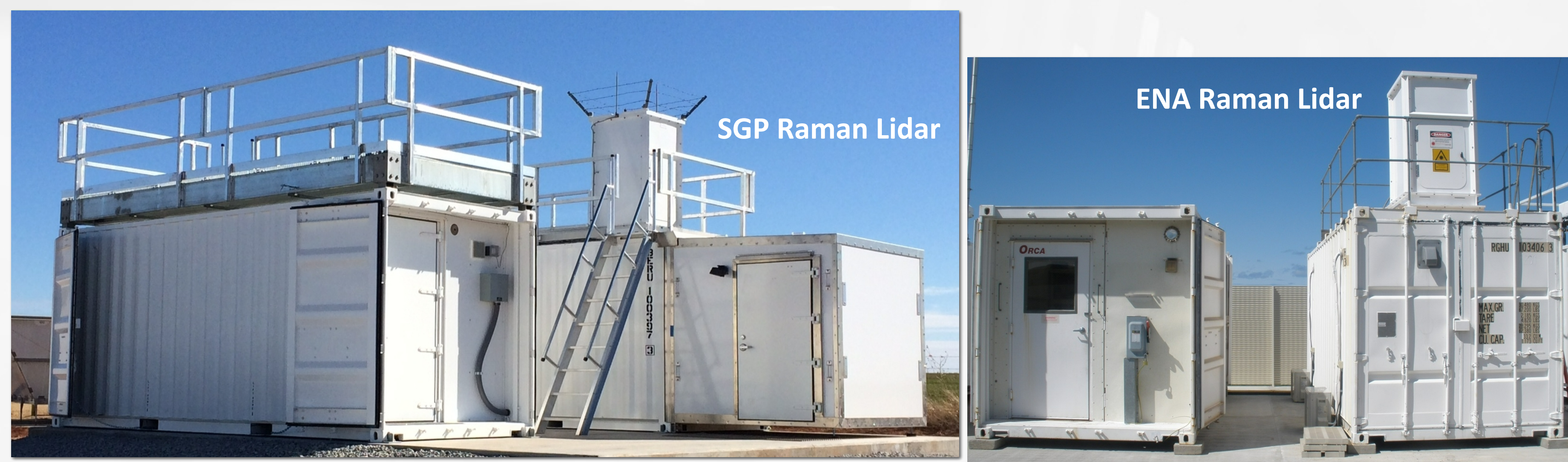
Fig. 1: Photos of two of the ARM Raman Lidars. The systems fill one sea container each with additional utilities in a separate container.
