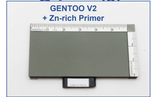
2 variants of GENTOO with and without Zn-rich primer to provide a durable ceramic hybrid inorganic/polymer coating with/without galvanic protection
