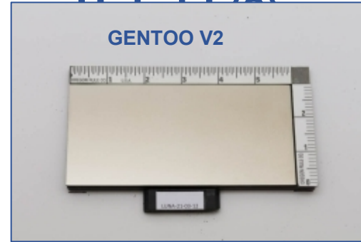
2 variants of GENTOO with and without Zn-rich primer to provide a durable ceramic hybrid inorganic/polymer coating with/without galvanic protection
