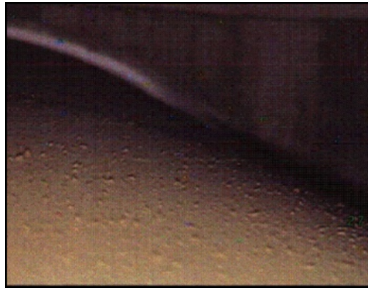
Dust on a storage canister surface, Calvert Cliffs ISFSI (EPRI 2014)
