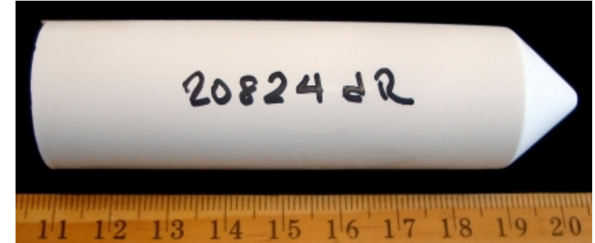
1:1 \text{CaSiO}_3 / \text{CaAl}_4\text{O}_7 with (\text{NaPO}_3)_6
