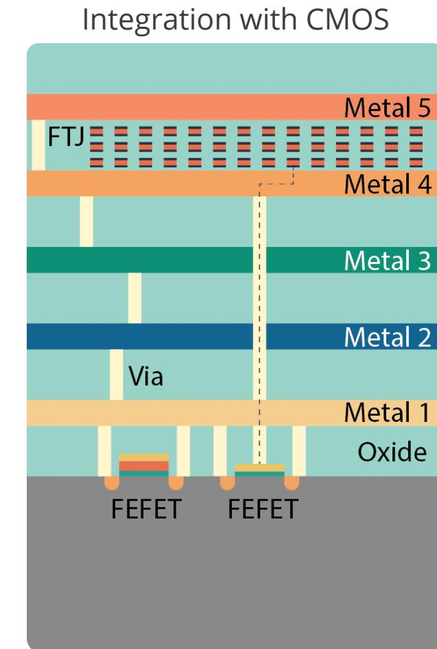
FeFET: ferroelectric field effect transistor
