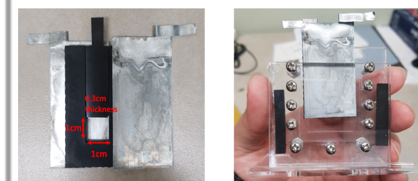
Figure 1. Experiment setup for Zn foil EIS measurement. The gel electrolyte was put into the square area from the top of the rubber gasket. Then, each Zn foil was assembled
