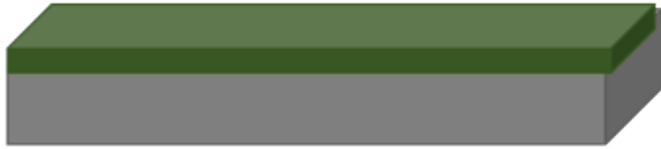
10 minute Ar plasma etch, mount in epoxy
