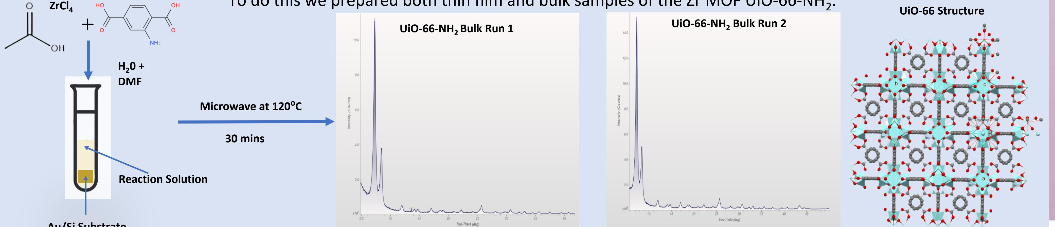
This reaction synthesized zirconium and 2-aminoterephthalic acid. The synthesis of UiO-66-NH<sub>2</sub> yields two products, a thin film and the bulk product.<sup>4</sup> A substrate consisting of a silicon substrate with a gold coating is placed in the vial and a thin film of UiO-66-NH<sub>2</sub> forms on the substrate. The bulk product is formed in a microwave vial along with the thin film. We set the temperature for 120°C for 30 mins and the synthesis is run in the microwave.
