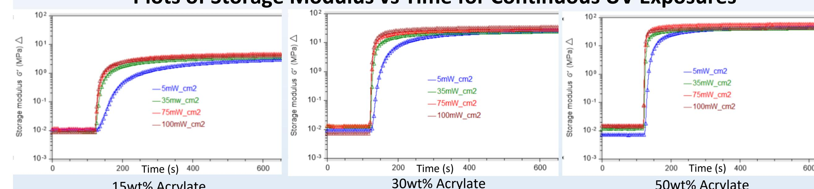
With photorheology we can see how using different UV intensities effects the cure kinetics and final modulus of each of our wt% formulations. Each test is run with a 25 min continuous UV exposure.
