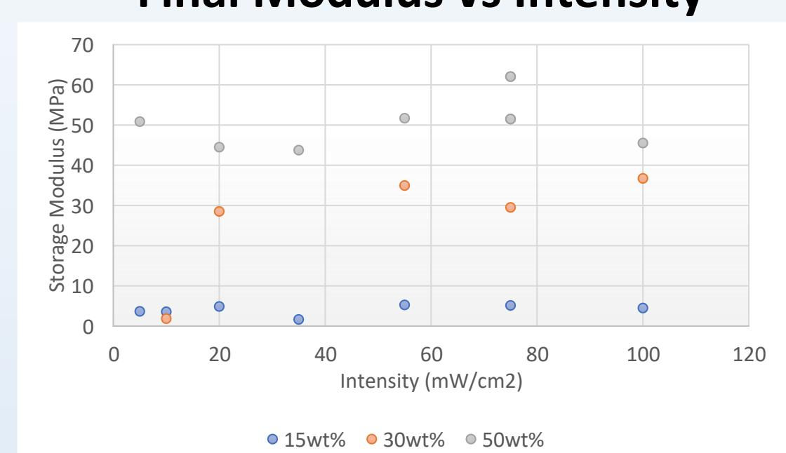
The final modulus after 25 min continuous UV exposure increases with increasing wt% acrylate.
