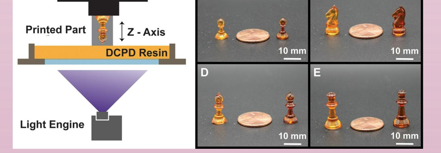
VP printing enables printing of parts with much higher resolution than DIW. Pieces on the left were VP printed with benzil/Ru-11 and on right with benzil/Ru-10.
