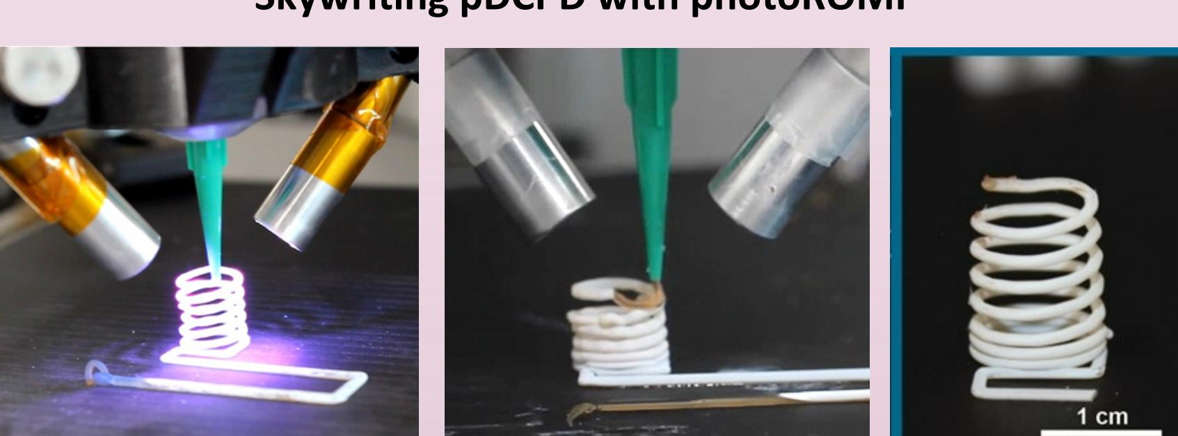
Turning UV on and off during free space printing shows that the ROMP is photocontrolled, and not a photoinitiated frontal polymerization (FRMP).
