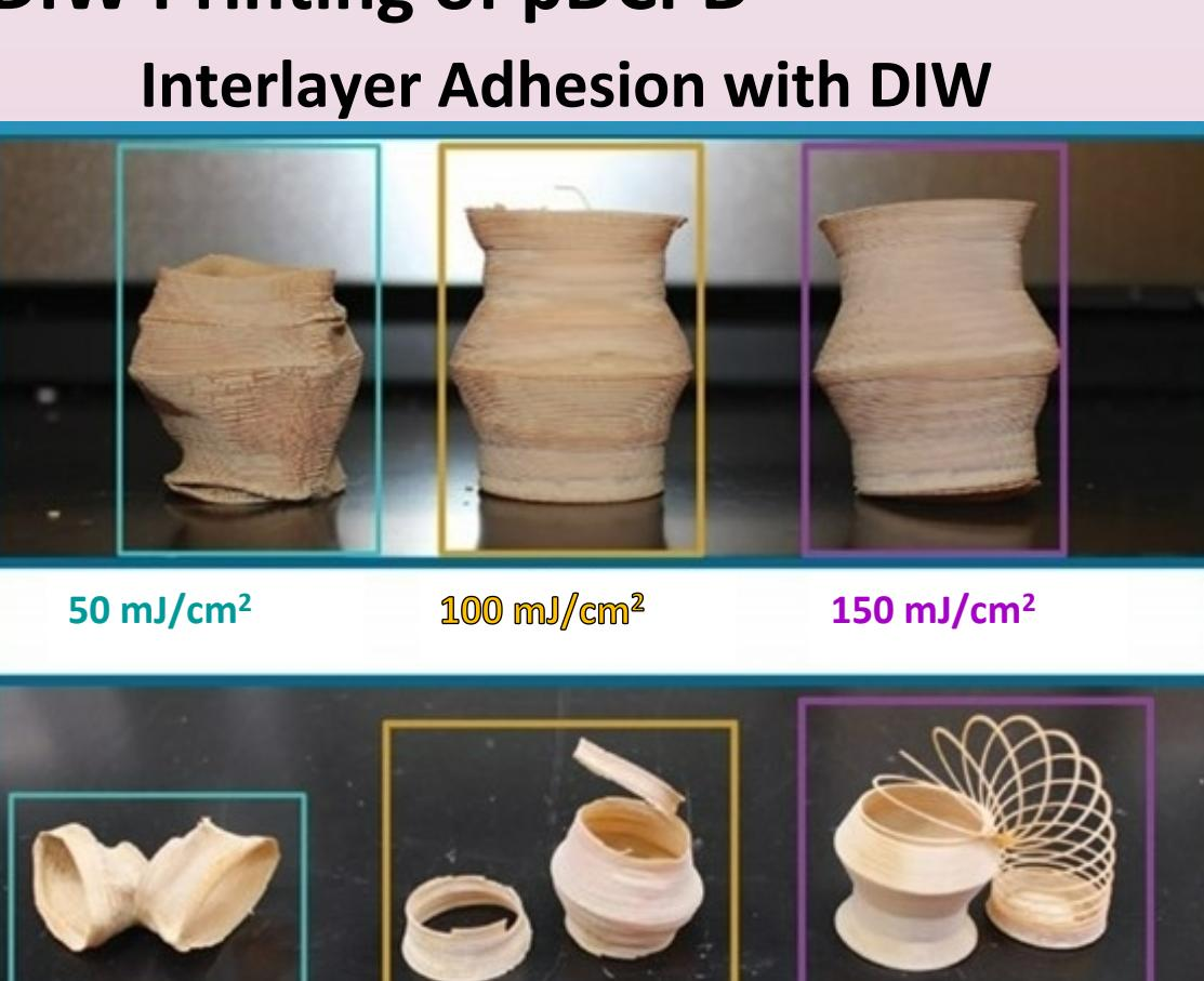
To the left is an example of the effects of interlayer adhesion during printing via DIW. The far left shows too low a UV dose which made the part not able to hold its own weight. The far right is an example of too high a UV dose which led to no interlayer adhesion, creating the slinky effect. The middle is an example of strong interlayer adhesion with a failure that does not occur along an interlayer boundary.
