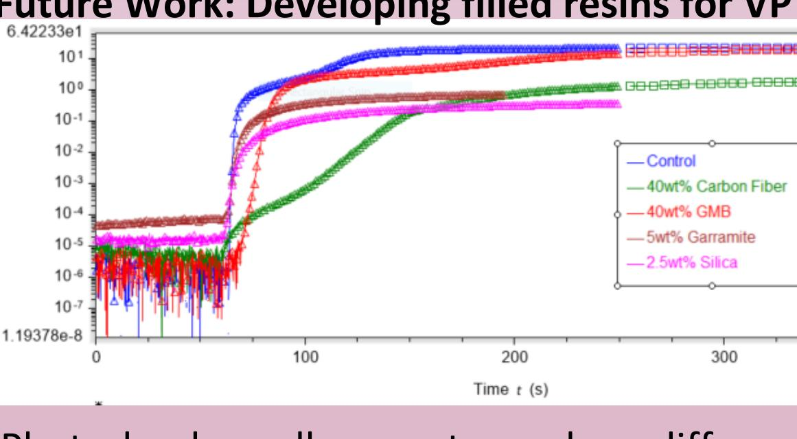
Photorheology allows us to see how different fillers impact our printable resin formulations.
