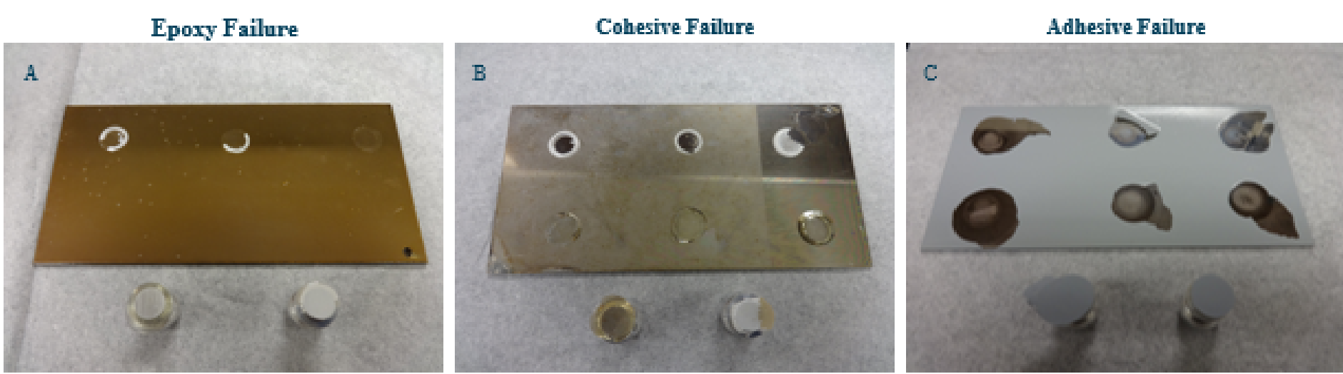
Figure 2. Exhibited failure during adhesion testing following 90-day exposure to salt and humidity.
