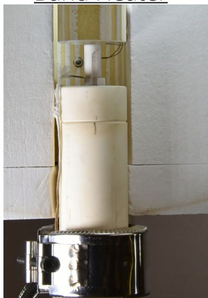
Quartz Top Alumina Bottom Band Heater
